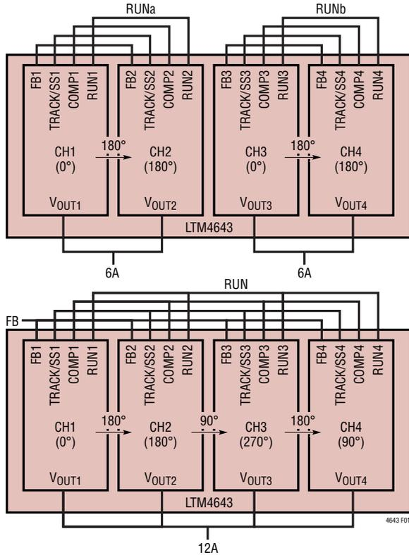
Figure 1. 2+2 and 4 Channels Parallel Concept Schematic
