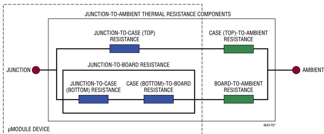
Figure 7. Graphical Representation of JEDEC 51-12 Thermal Coefficients
