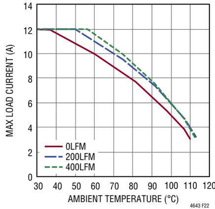
**Figure 22. 5V<sub>IN</sub> to 3.3V<sub>OUT</sub> Derating Curve, 4-Channel Paralleled, No Heat Sink**
