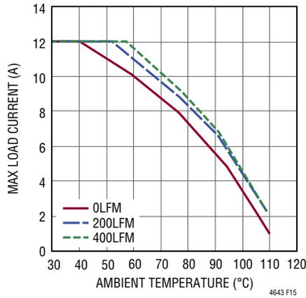
**Figure 15. 12V<sub>IN</sub> to 1.0V<sub>OUT</sub> Derating Curve, 4-Channel Paralleled, No Heat Sink**
