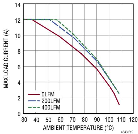
**Figure 19. 12V<sub>IN</sub> to 1.5V<sub>OUT</sub> Derating Curve, 4-Channel Paralleled, No Heat Sink**
