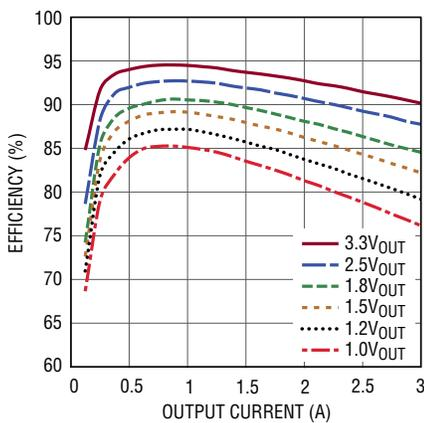
**Efficiency vs Load Current from 12V<sub>IN</sub> (One Channel Operating)**
