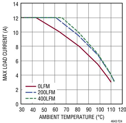
**Figure 24. 5V<sub>IN</sub> to 3.3V<sub>OUT</sub> Derating Curve, 4-Channel Paralleled, BGA Heat Sink**
