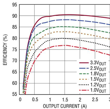
**DCM Mode Efficiency from 1.5V<sub>OUT</sub>**
