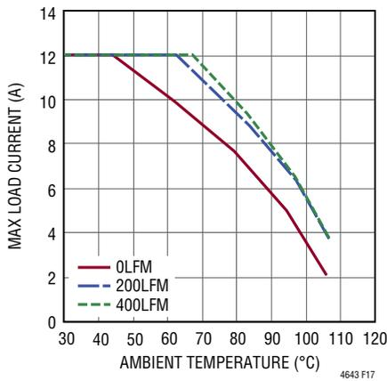
**Figure 17. 12V<sub>IN</sub> to 1.0V<sub>OUT</sub> Derating Curve, 4-Channel Paralleled, BGA Heat Sink**
