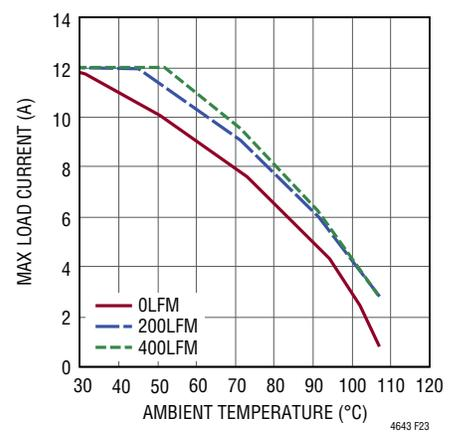
**Figure 23. 12V<sub>IN</sub> to 3.3V<sub>OUT</sub> Derating Curve, 4-Channel Paralleled, No Heat Sink**
