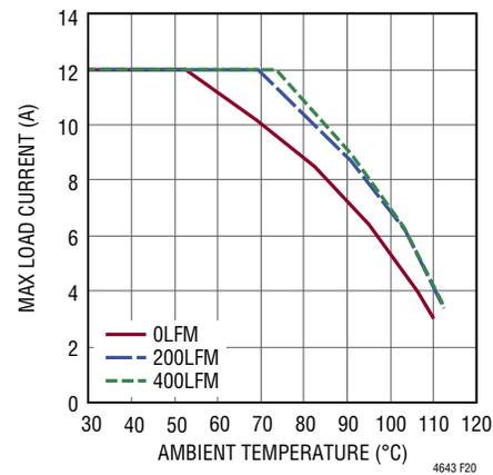
**Figure 20. 5V<sub>IN</sub> to 1.5V<sub>OUT</sub> Derating Curve, 4-Channel Paralleled, BGA Heat Sink**
