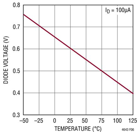
Figure 6. Diode Voltage  $V_D$  vs Temperature  $T(^{\circ}C)$
