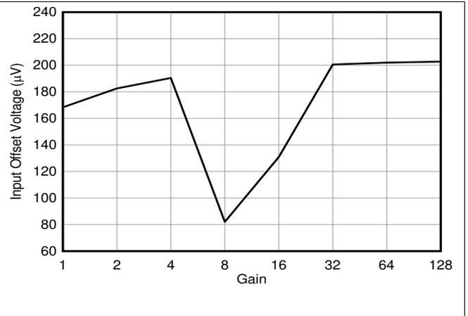
Figure 5. Input Offset Voltage vs Gain
