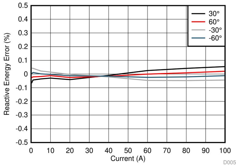
**Figure 103. Cumulative Reactive Energy % Error Versus Current**
