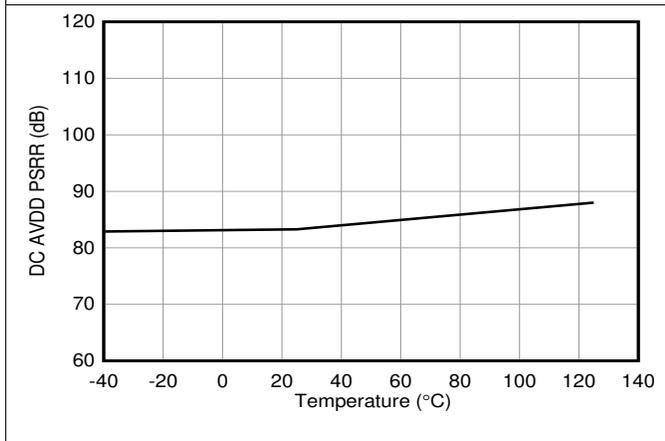
Figure 8. DC AVDD PSRR vs Temperature
