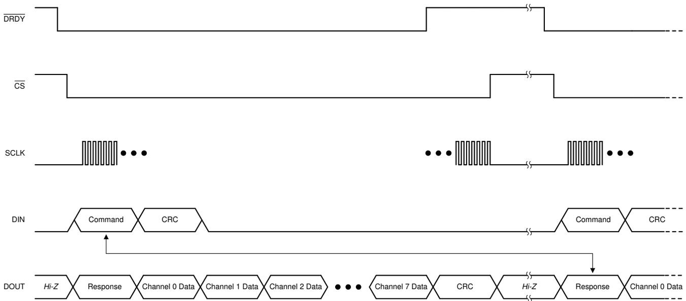
**Figure 36. Typical Communication Frame**
