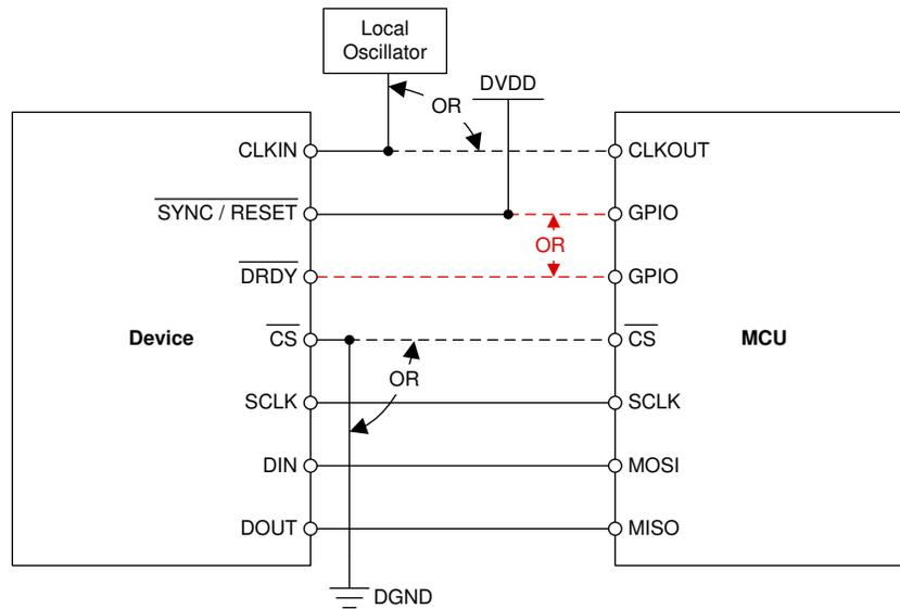
Figure 96. Minimum Connections Required to Operate the ADS131M08
