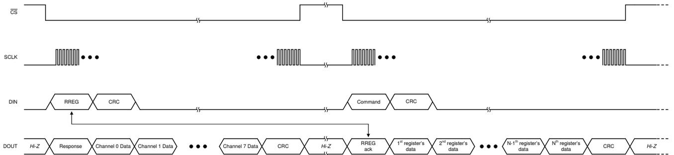
Figure 42. Reading Multiple Registers
