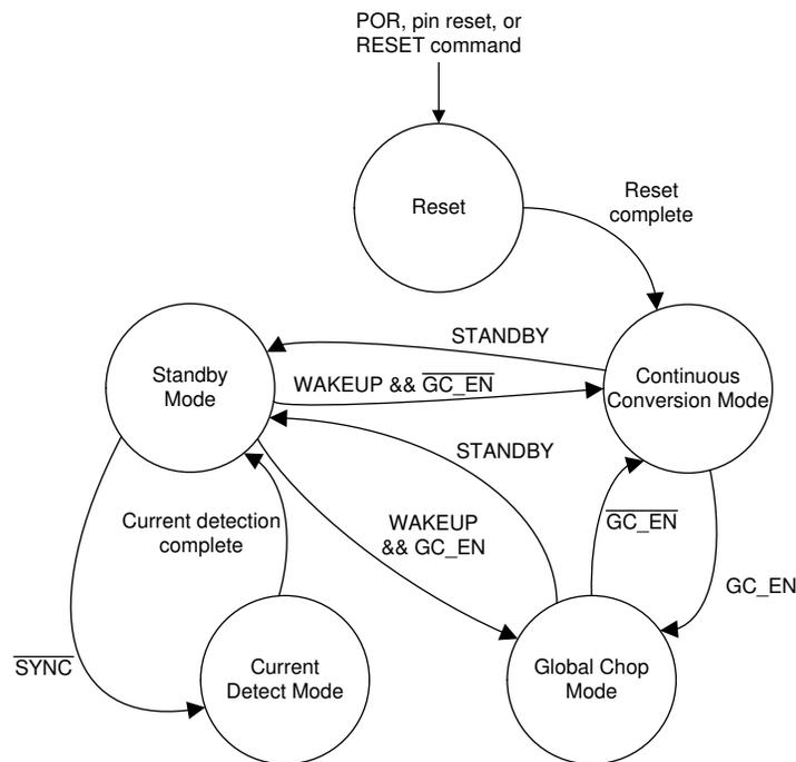
**Figure 34. State Diagram Depicting Device Functional Modes**
