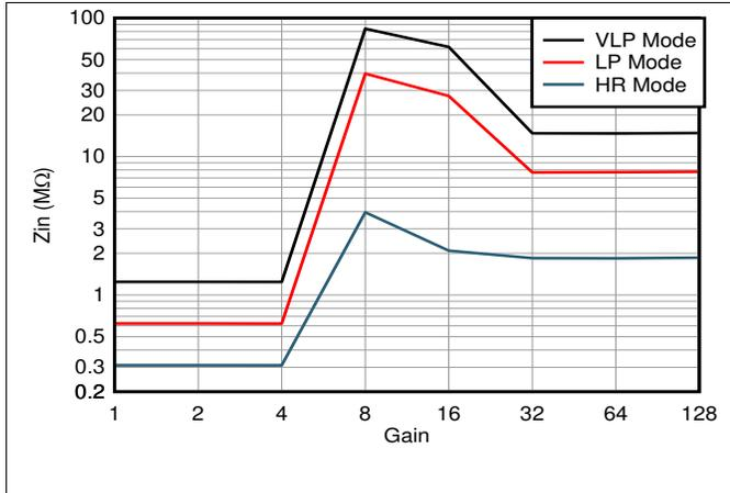
Figure 4. Input Impedance vs Gain
