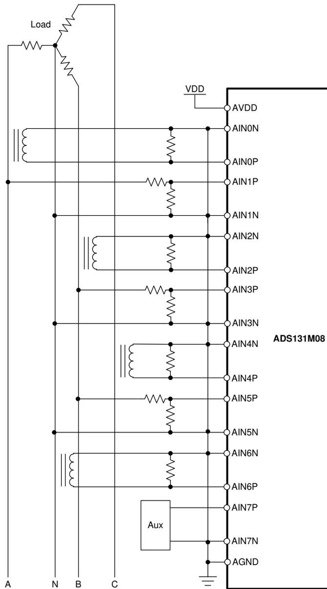
**Figure 97. Three-Phase Current and Voltage Measurement Front-End With a Neutral Current Monitor**
