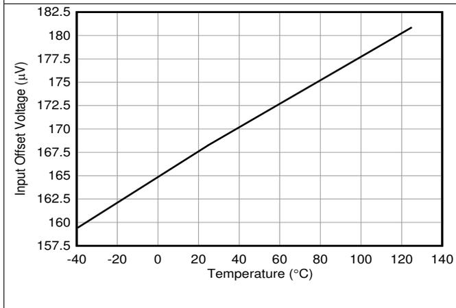
Figure 6. Input Offset Voltage vs Temperature
