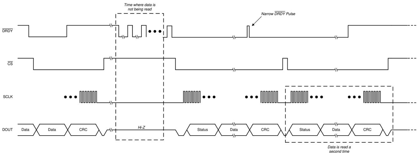
**Figure 39. Collecting Data After a Hiatus by Reading Data Twice**
