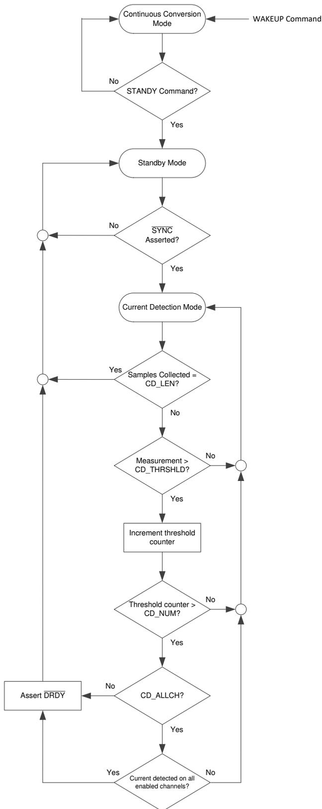
Figure 35. Current-Detect Mode Flow Chart
