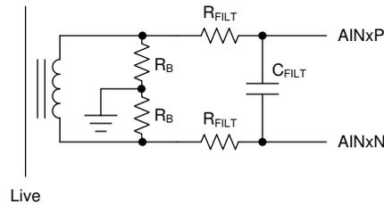
**Figure 101. Current Measurement Front-End**
