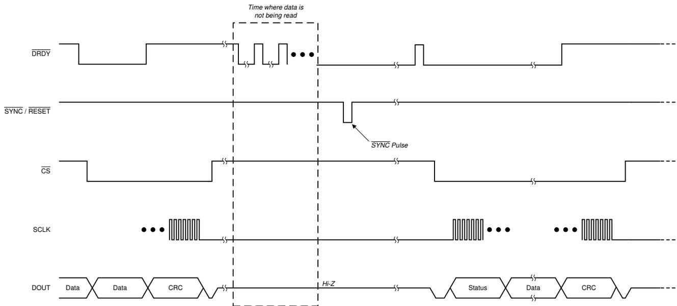
**Figure 38. Collecting Data After a Hiatus Using the  $\overline{\text{SYNC/RESET}}$  Pin**
