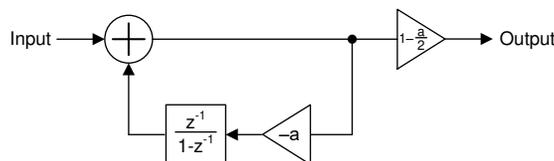
**Figure 28. DC Block Filter Topology**
