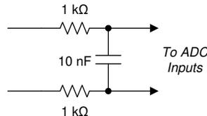
**Figure 95. Recommended Antialiasing Circuitry**
