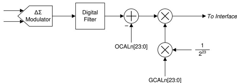
**Figure 32. Calibration Block Diagram**
