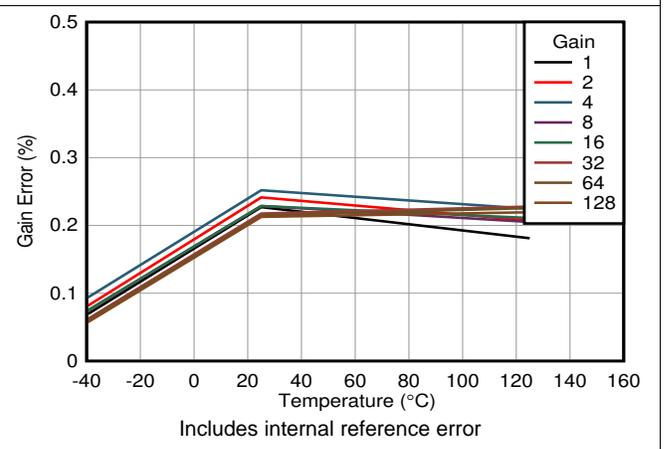
Figure 7. Gain Error vs Temperature
