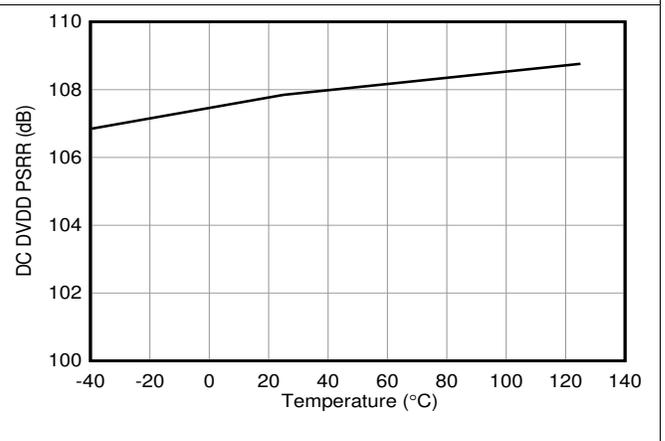
Figure 9. DC DVDD PSRR vs Temperature
