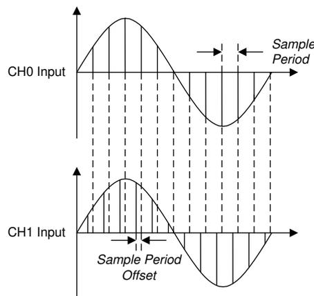
**Figure 30. Channel 1 With a Positive Sample Phase Shift With Respect to Channel 0**
