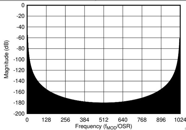
Figure 24. Sinc<sup>3</sup> Digital Filter Response, OSR 1024, Stop-Band Detail
