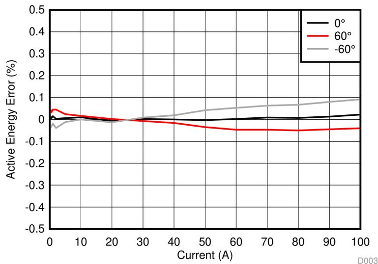
**Figure 102. Cumulative Phase Active Energy % Error Versus Current**
