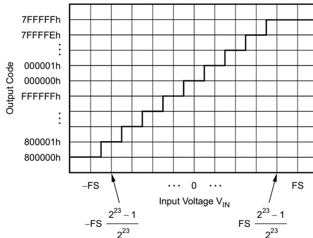
Figure 37. Code Transition Diagram
