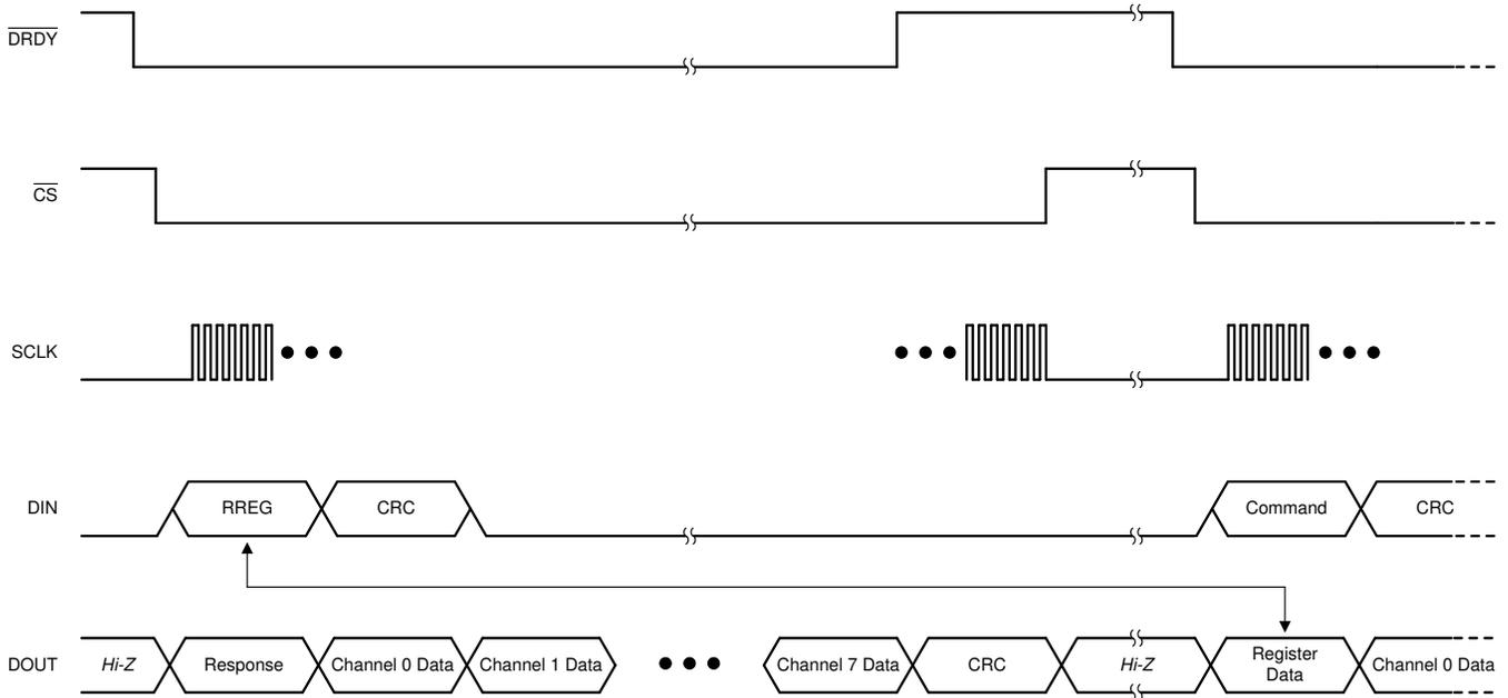
Figure 41. Reading a Single Register
