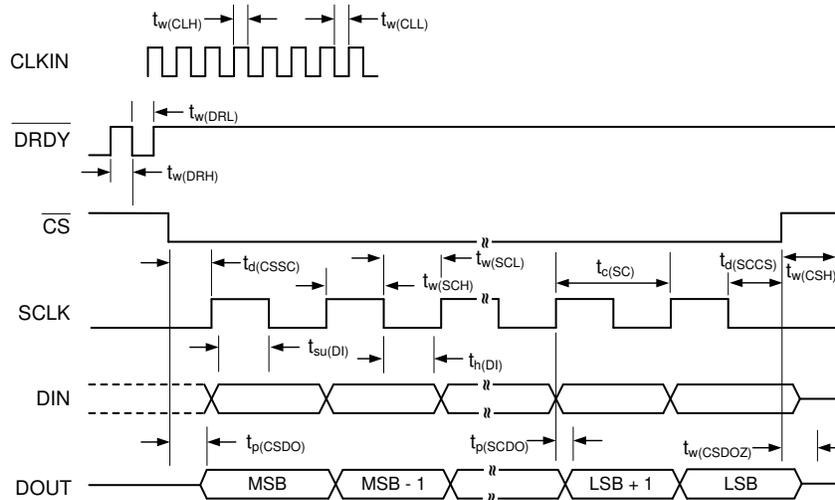
NOTE: SPI settings are CPOL = 0 and CPHA = 1.  $\overline{CS}$  transitions must take place when SCLK is low.
