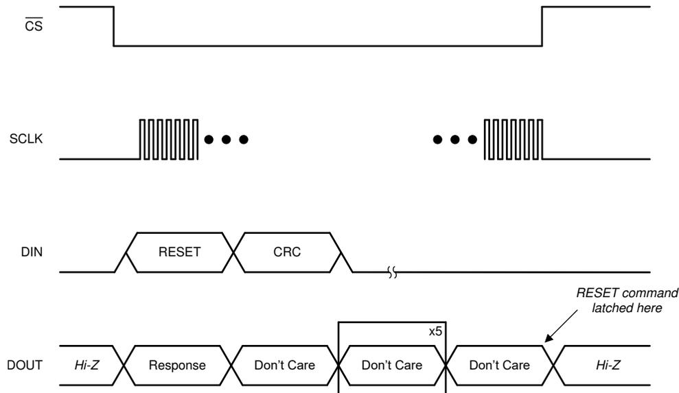
**Figure 40. RESET Command Frame**
