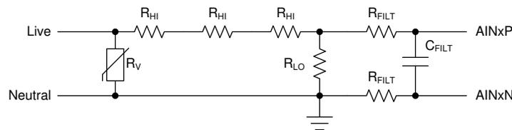
**Figure 100. Voltage Measurement Front-End**
