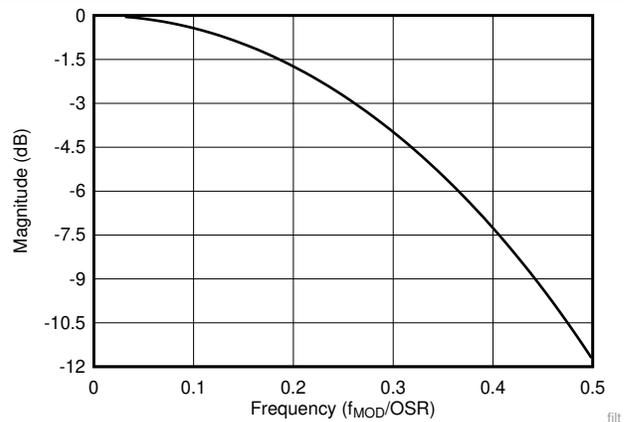
Figure 23. Sinc<sup>3</sup> Digital Filter Response, Pass-Band Detail
