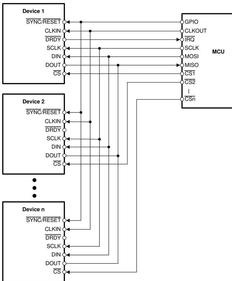
Figure 98. Multiple Device Configuration
