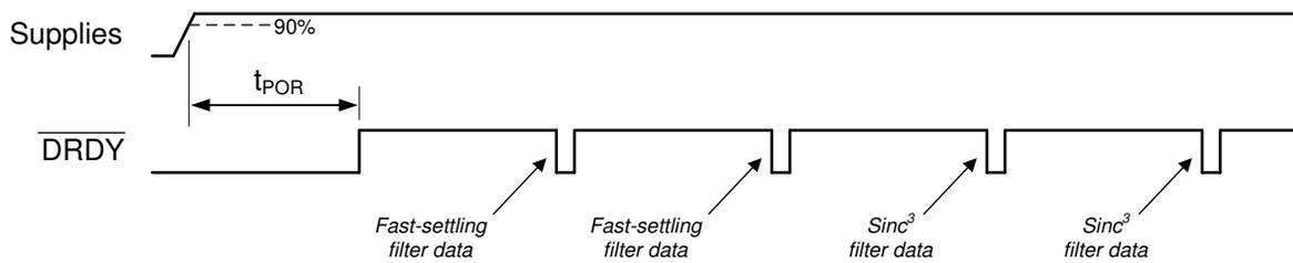
Figure 33. Fast-Settling Behavior
