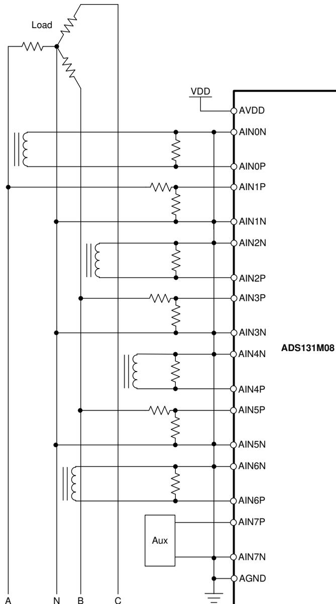
Figure 99. Three-Phase Metrology Design Front-End
