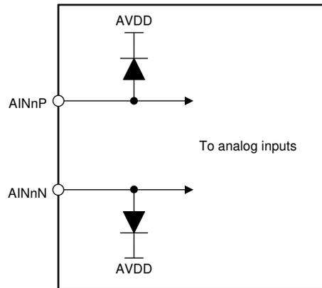
**Figure 20. Input ESD Protection Circuitry**
