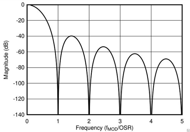
Figure 22. Sinc<sup>3</sup> Digital Filter Response
