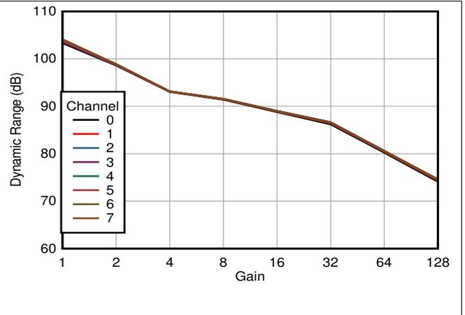
Figure 11. Dynamic Range vs Gain across Channels
