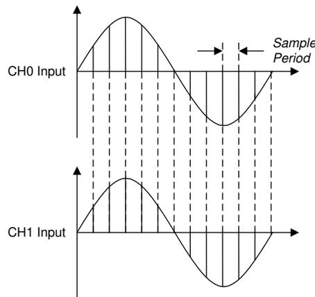
**Figure 29. Two Channel Outputs With Equal Phase Settings**
