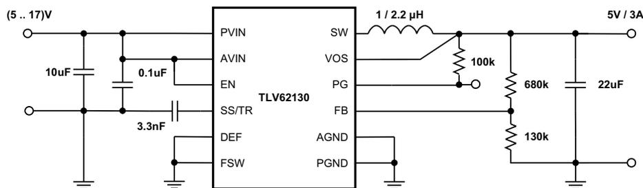
Figure 41. 5-V / 3-A Power Supply
