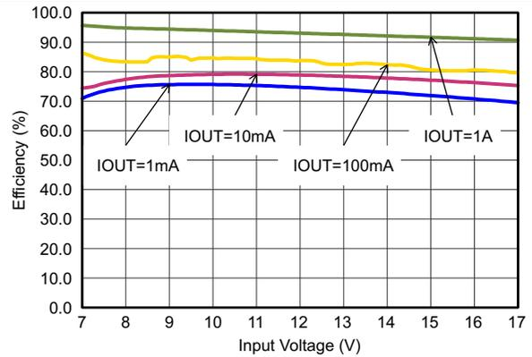
**Figure 11. Efficiency With 2.5 MHz, Vout = 5 V**
