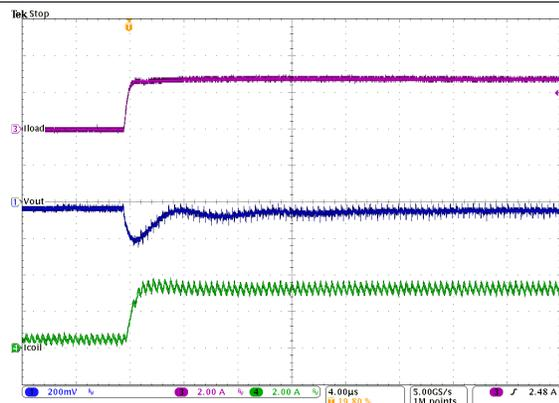
Figure 30. Load Transient Response of Figure 29,
