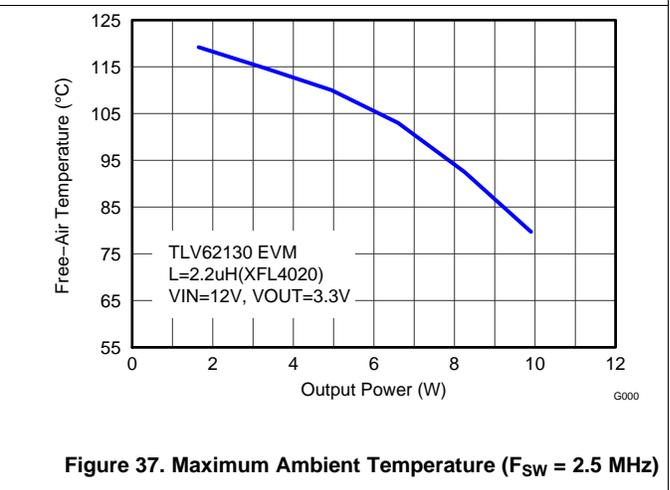
Figure 37. Maximum Ambient Temperature ( $F_{SW} = 2.5\text{ MHz}$ )
