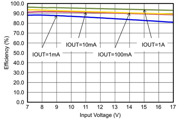
**Figure 9. Efficiency With 1.25 MHz, Vout = 5 V**
