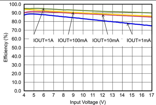
**Figure 13. Efficiency With 1.25 MHz, Vout = 3.3 V**
