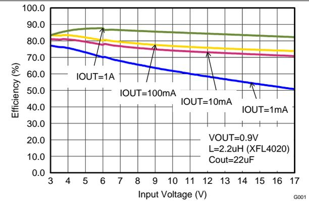
Figure 19. Efficiency With 1.25 MHz,  $V_{out} = 0.9\text{ V}$
