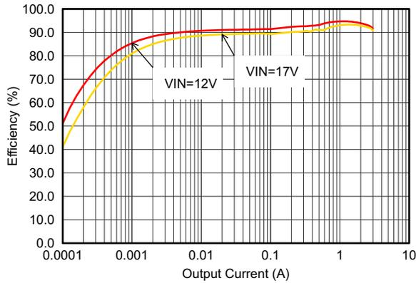
**Figure 8. Efficiency With 1.25 MHz, Vout = 5 V**
