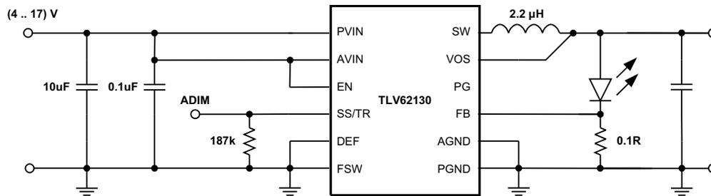
**Figure 38. 3 A Single LED Power Supply**
