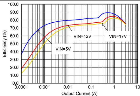
Figure 18. Efficiency With 1.25 MHz,  $V_{out} = 0.9\text{ V}$
