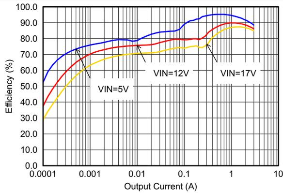
Figure 14. Efficiency With 2.5 MHz,  $V_{out} = 3.3\text{ V}$
