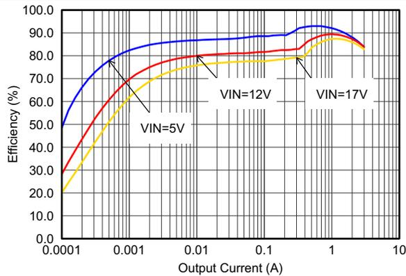
Figure 16. Efficiency With 1.25 MHz,  $V_{out} = 1.8\text{ V}$
