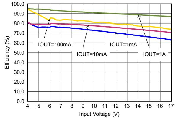
Figure 15. Efficiency With 2.5 MHz,  $V_{out} = 3.3\text{ V}$
