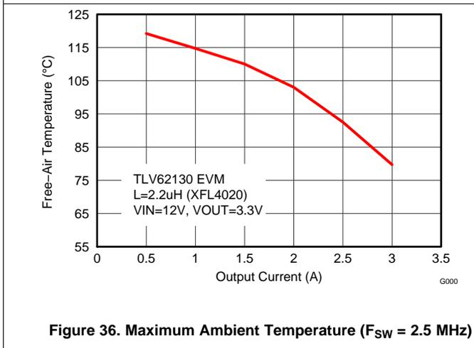
Figure 36. Maximum Ambient Temperature ( $F_{SW} = 2.5\text{ MHz}$ )
