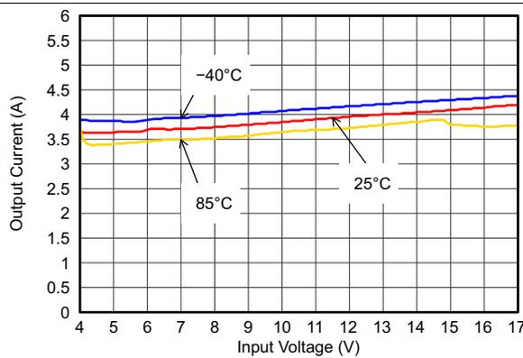
Figure 25. Maximum Output Current
