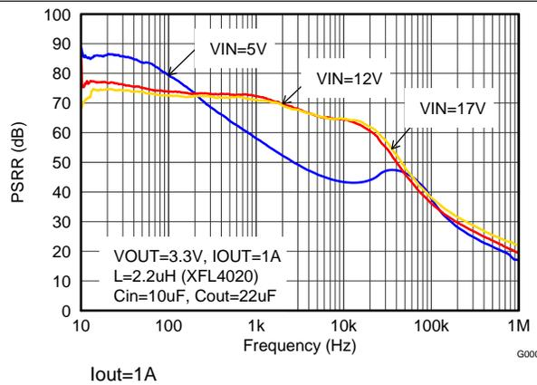
Figure 26. Power Supply Rejection Ratio,  $F_{SW} = 2.5\text{ MHz}$
