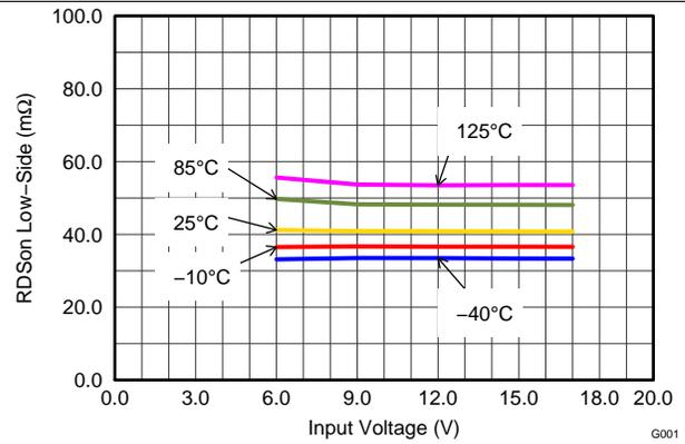
Figure 4. Low-Side Switch Resistance
