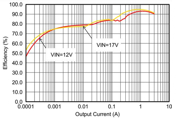
**Figure 10. Efficiency With 2.5 MHz, Vout = 5 V**
