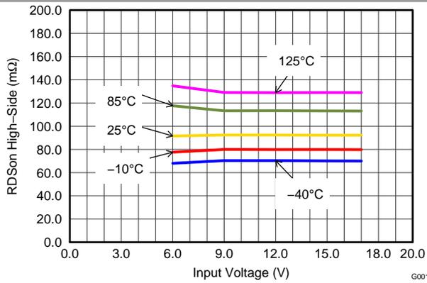
Figure 3. High-Side Switch Resistance
