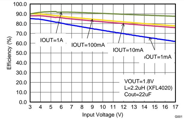
Figure 17. Efficiency With 1.25 MHz,  $V_{out} = 1.8\text{ V}$
