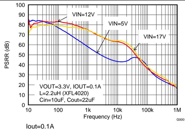
Figure 27. Power Supply Rejection Ratio,  $F_{SW} = 2.5\text{ MHz}$
