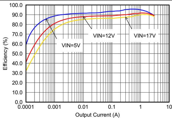
**Figure 12. Efficiency With 1.25 MHz, Vout = 3.3 V**
