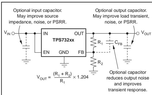
**Figure 33. Typical Application Circuit for Adjustable-Voltage Versions**
