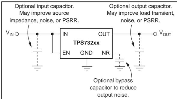
**Figure 32. Typical Application Circuit for Fixed-Voltage Versions**
