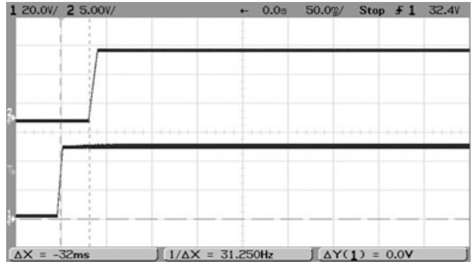
Stepload Transient Response (Vin = 48V, Iout = 50-75-50% of Iout, Load = 1uF || 10uF,
