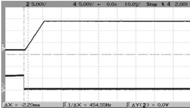
Startup Delay (Vin = 48V, Iout = 35A, Cout = 1000uF, Ta = +25°C)
