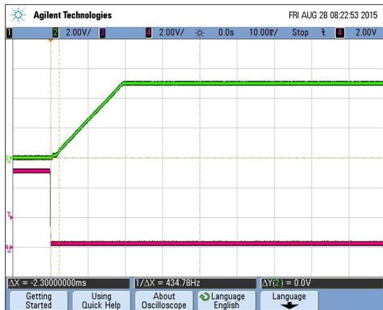
Startup Delay (Vin = 48V, Iout = 60A, Cload = 1000uF, Ta = +25°C)
