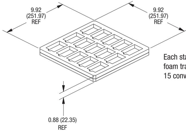
Each static dissipative polyethylene foam tray accommodates 15 converters in a 3 x 5 array.
