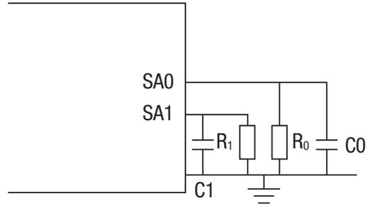
Figure 1. Schematic of Connection of Address Resistors
