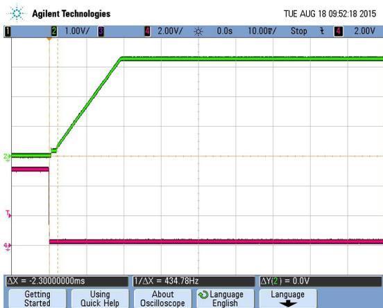
Startup Delay (Vin = 48V, Iout = 60A, Cloud = 1000uF, Ta = +25°C)
