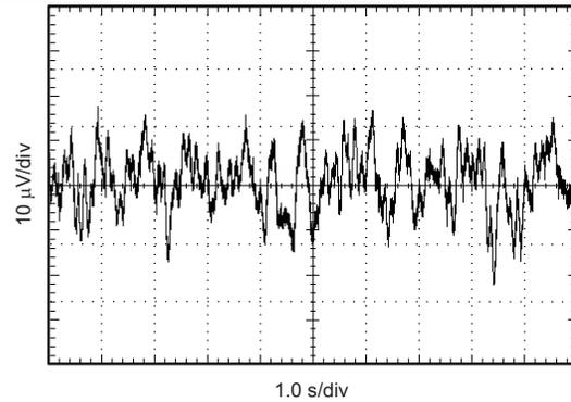
Figure 20. 0.1-Hz to 10-Hz Noise
