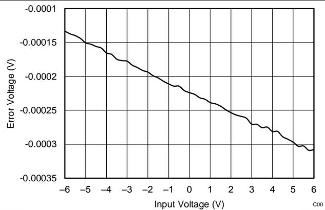
Figure 32. OPA317 Output Voltage Error vs Input Voltage
