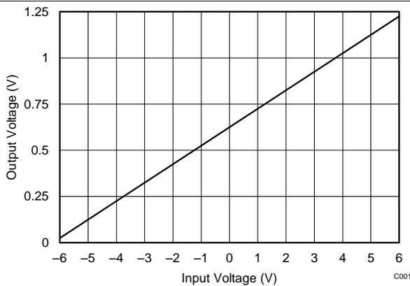
Figure 31. OPA317 Output Voltage vs Input Voltage
