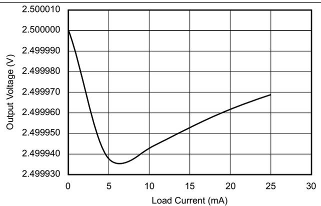
Figure 12. Output Voltage vs Load Current
