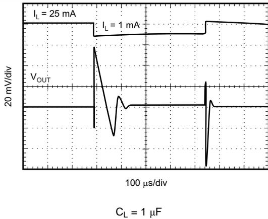
Figure 19. 1-mA to 25-mA Load Transient
