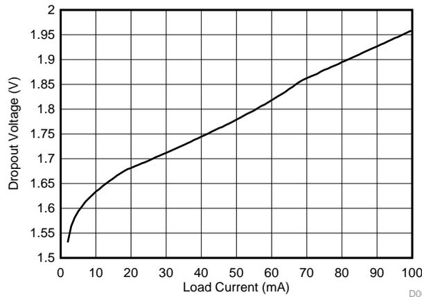
Figure 1. Dropout Voltage vs Load Current ( $T_J = 25^\circ\text{C}$ )
