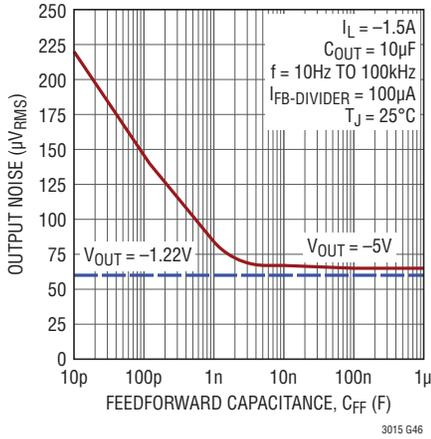
**LT3015 10Hz to 100kHz Output Noise**
