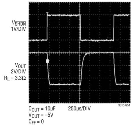
**SHDN Transient Response,  $I_L = -1.5\text{A}$ ,  $C_{FF} = 10\text{nF}$**
