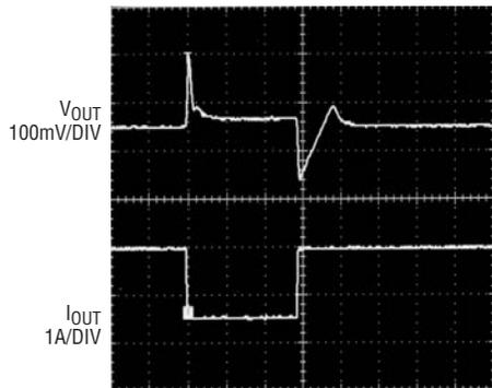
$C_{OUT} = 10\mu\text{F}$  25 $\mu\text{s}/\text{DIV}$
