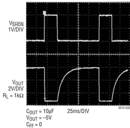
**SHDN Transient Response,  $I_L = -1.5\text{A}$ ,  $C_{FF} = 0$**
