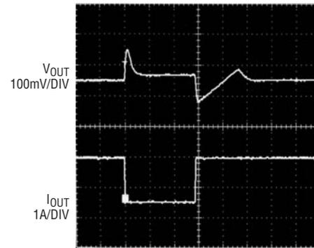
$C_{OUT} = 47\mu\text{F}$  25 $\mu\text{s}/\text{DIV}$
