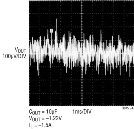
**LT3015 10Hz to 100kHz Output Noise,  $C_{FF} = 0$**
