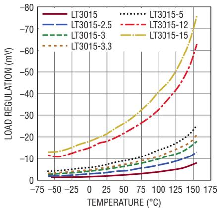
$V_{IN} = V_{OUT(NOMINAL)} - 1V$
