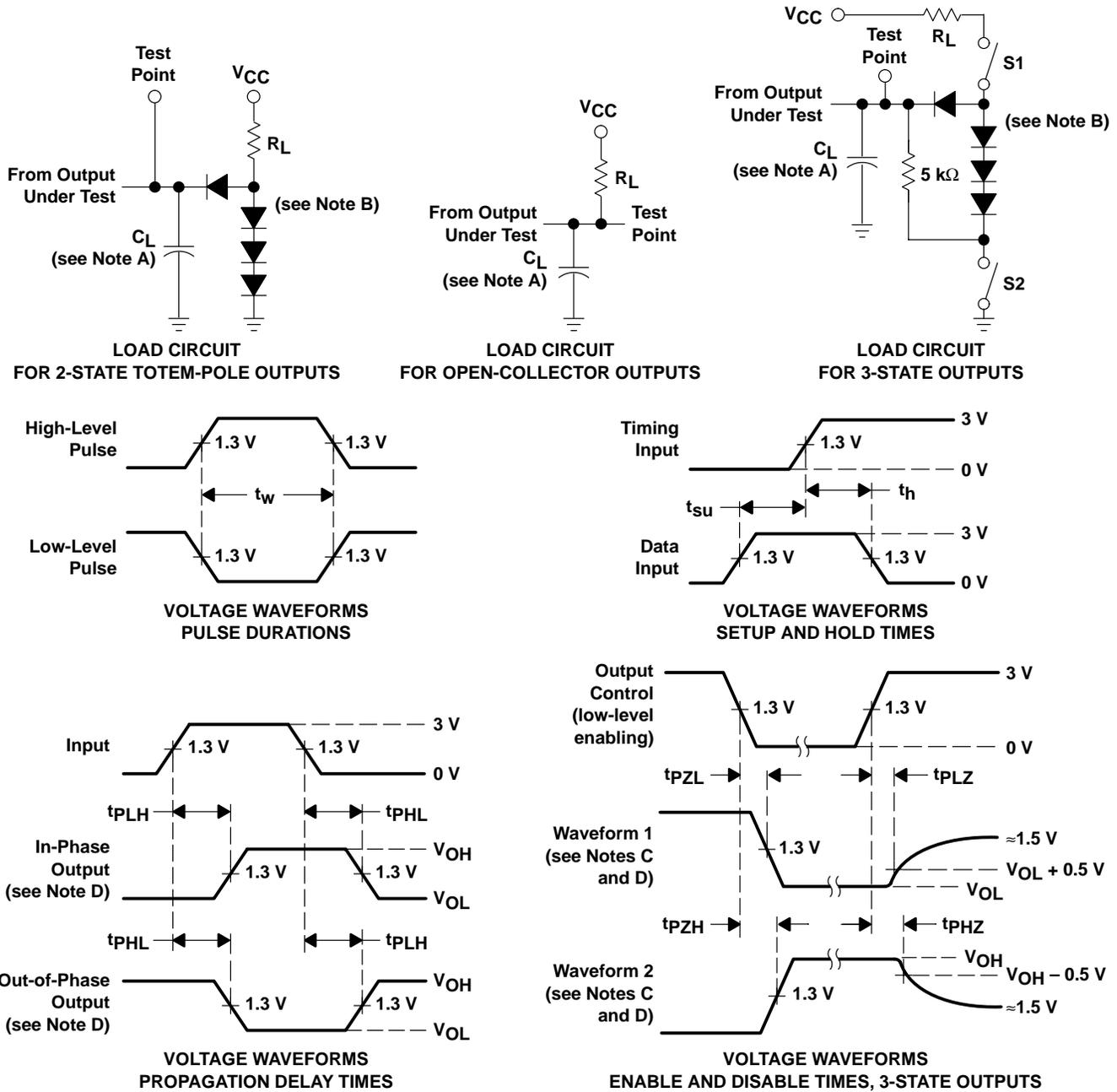
Figure 2. Load Circuits and Voltage Waveforms
