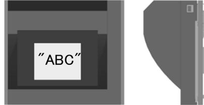
**Fig. 10. Display position at vflip=1, hflip=1**
