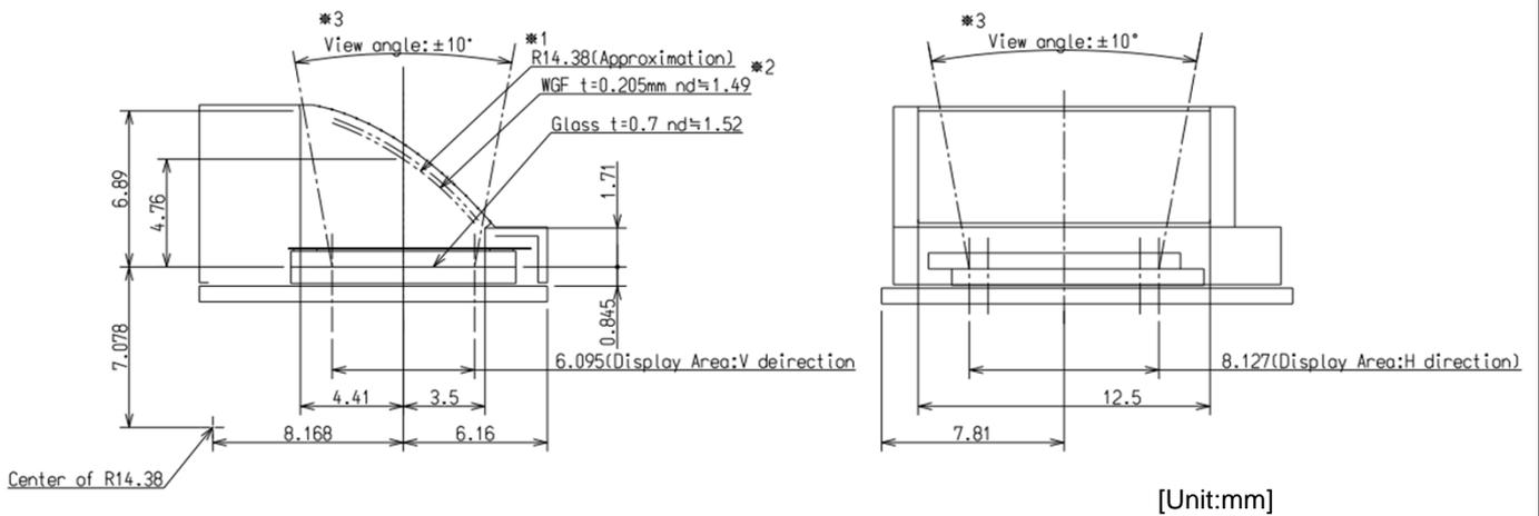
\*1 The cross-section curve of the WGF(Wire Grid Film) is not true circle and is confidential.
