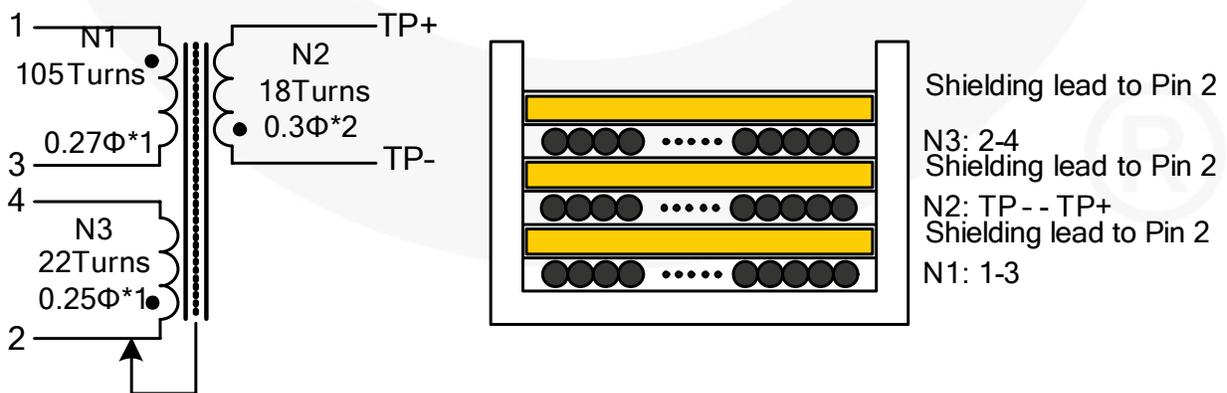
Figure 18. Transformer Structure
