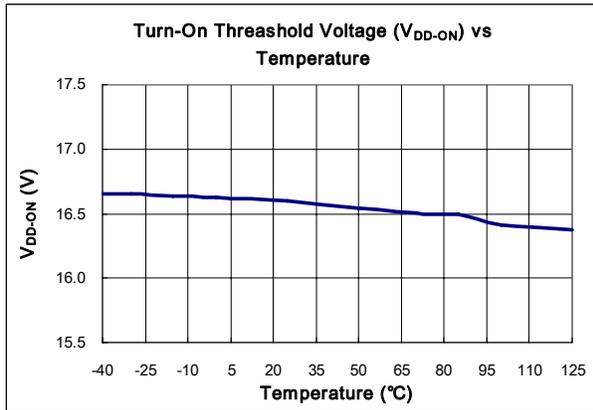
Figure 6. Turn-On Threshold Voltage (V<sub>DD-ON</sub>) vs. Temperature
