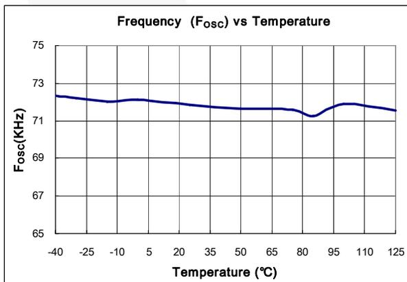
Figure 10. Frequency (f<sub>osc</sub>) vs. Temperature
