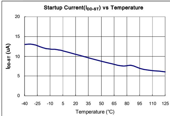
Figure 8. Startup Current (I<sub>DD-ST</sub>) vs. Temperature
