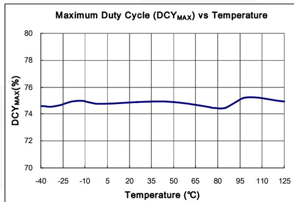
Figure 11. Maximum Duty Cycle (DCY<sub>MAX</sub>) vs. Temperature
