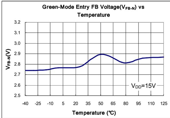
**Figure 12. Green Mode Entry FB Voltage (V<sub>FB-N</sub>) vs. Temperature**
