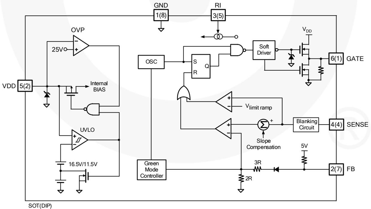
Figure 2. Block Diagram
