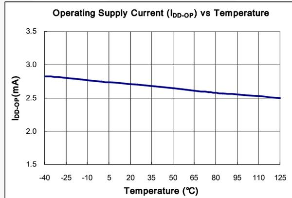
Figure 9. Operating Supply Current (I<sub>DD-OP</sub>) vs. Temperature
