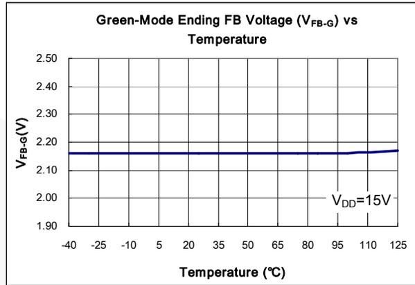
**Figure 13. Green Mode Ending FB Voltage (V<sub>FB-G</sub>) vs. Temperature**
