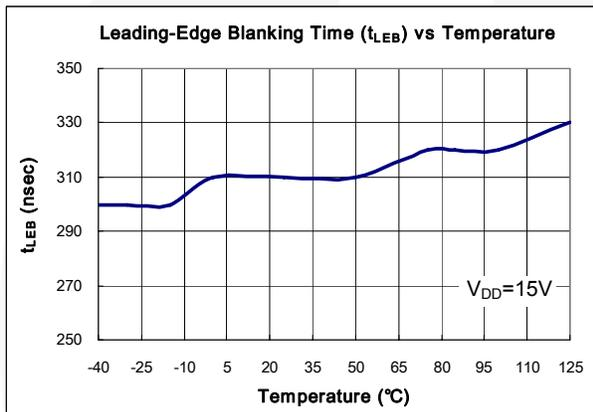
**Figure 14. Leading-Edge Blanking Time (t<sub>LEB</sub>) vs. Temperature**
