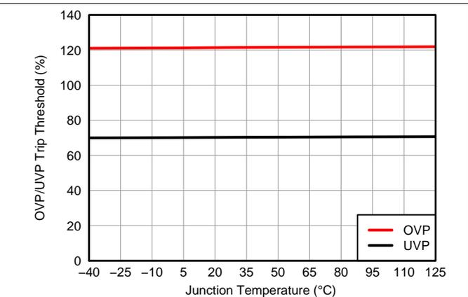
Figure 4. OVP/UVP Trip Threshold vs. Junction Temperature
