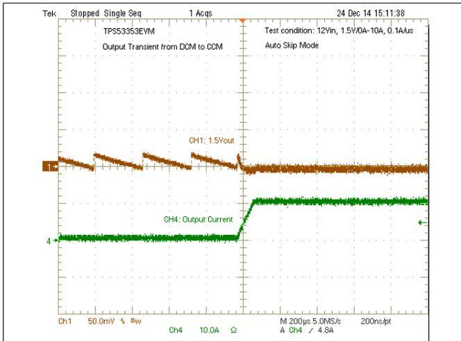
Figure 44. Output Transient from DCM to CCM
