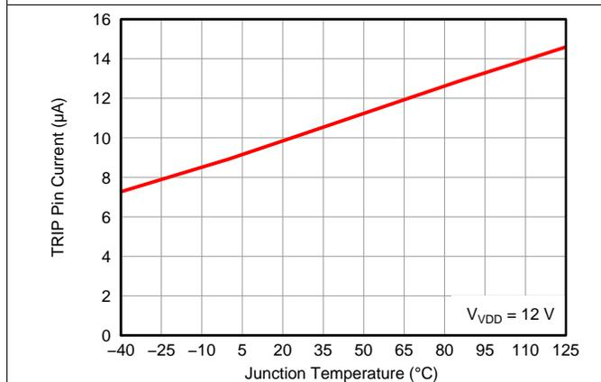
Figure 3. TRIP Pin Current vs. Junction Temperature
