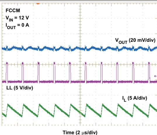
Figure 17. 1.1-V Output FCCM Mode Steady-State Operation
