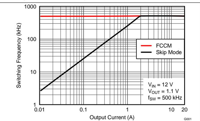
Figure 6. Switching Frequency vs. Output Current
