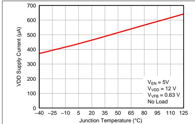
Figure 1. VDD Supply Current vs. Junction Temperature
