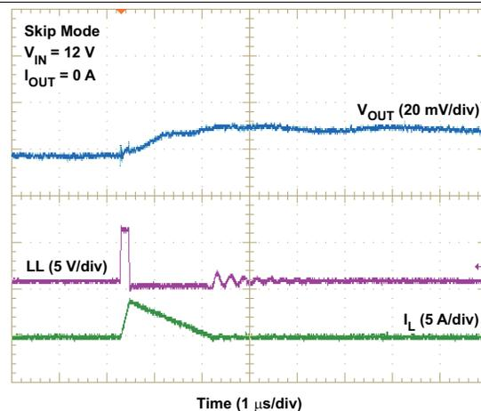
Figure 18. 1.1-V Output Skip Mode Steady-State Operation
