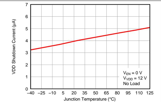
Figure 2. VDD Shutdown Current vs. Junction Temperature
