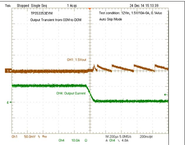
Figure 45. Output Transient from CCM to DCM
