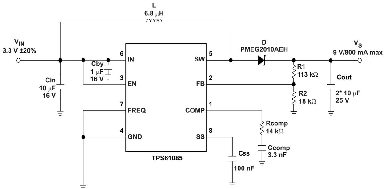
Figure 15. Typical Application, 3.3 V to 9 V ( $f_{sw} = 650$  kHz)
