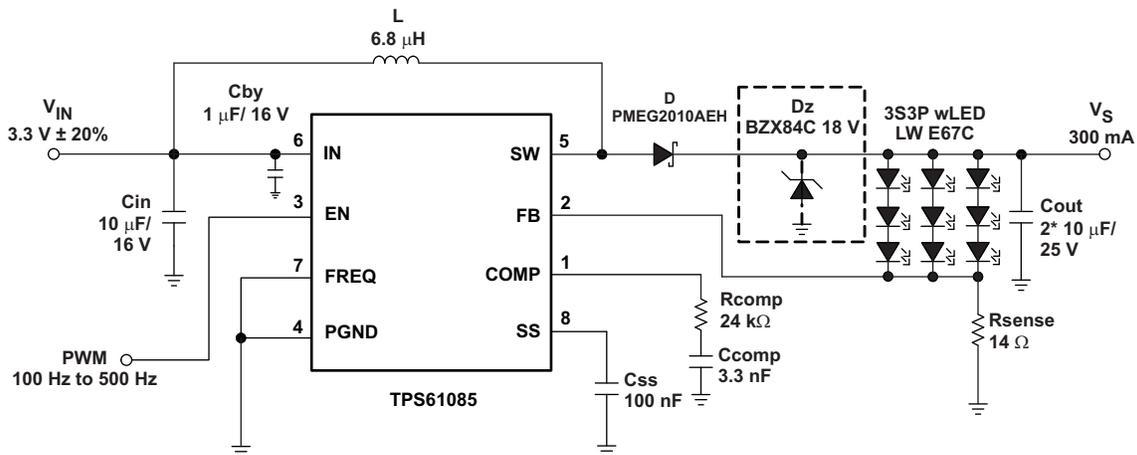
Figure 19. Simple Application (3.3V input -  $f_{sw} = 650\text{ kHz}$ ) for wLED Supply (3S3P) with Adjustable Brightness Control using a PWM Signal on the Enable Pin (with optional clamping Zener diode)
