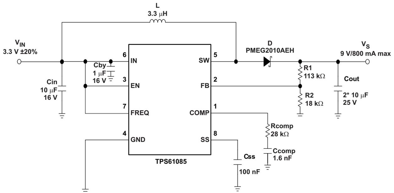
Figure 14. Typical Application, 3.3 V to 9 V ( $f_{sw} = 1.2$  MHz)
