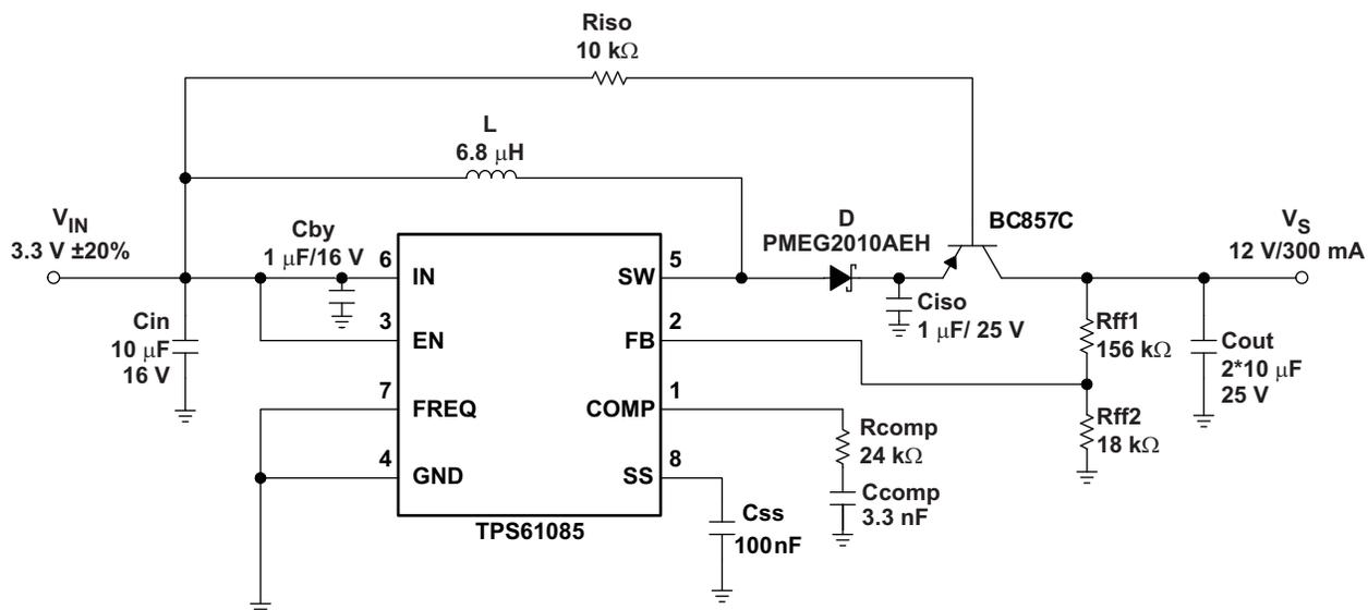
Figure 16. Typical Application with External Load Disconnect Switch
