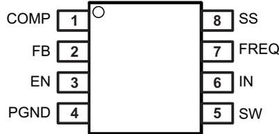
8-PIN 4.9mm x 3mm x 1.1mm MSOP (DGK)
