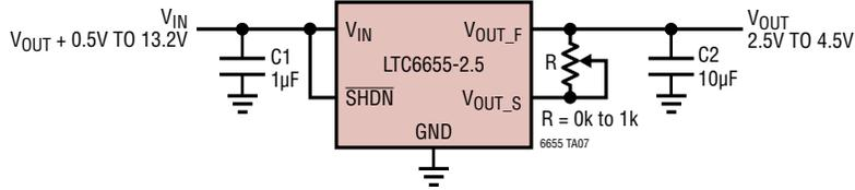
$V_{OUT} = \text{VOLTAGE OPTION} + 0.002 \cdot R$
