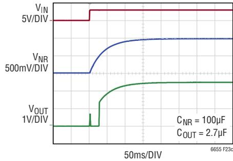
Figure 23c.  $C_{NR} = 100\mu\text{F}$
