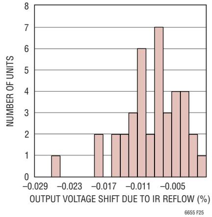
Figure 25. Output Voltage Shift Due to IR Reflow
