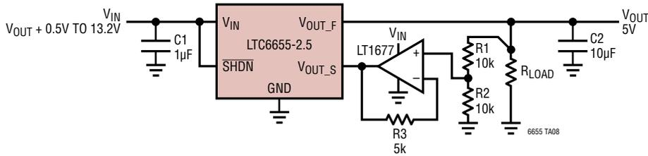
$V_{OUT} = \text{VOLTAGE OPTION} \cdot (1 + R1/R2)$
