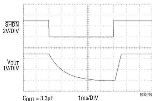
Figure 8. Shutdown Response with 5mA Source Load
