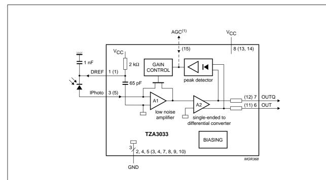
(1) AGC analog I/O is only available on the TZA3033U (pad 15). The numbers in brackets refer to the pad numbers of the naked die version.
