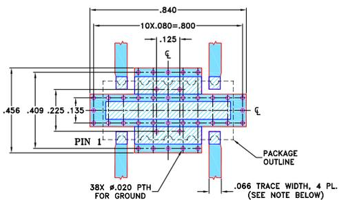
NOTE: 1. TRACE WIDTH IS SHOWN FOR ROGERS R04350B WITH DIELECTRIC THICKNESS .030"±.002"; COPPER: 1/2 OZ. EACH SIDE. FOR OTHER MATERIALS TRACE WIDTH MAY NEED TO BE MODIFIED.
