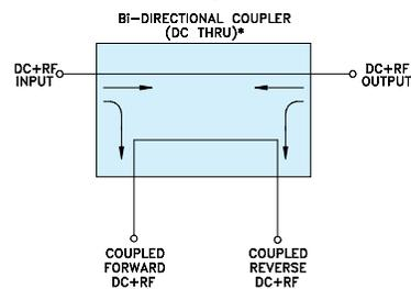
\* ELECTRICAL SCHEMATIC IS FOR BI-DIRECTIONAL COUPLER WITHOUT INTERNAL TRANSFORMERS AND RESISTORS.
