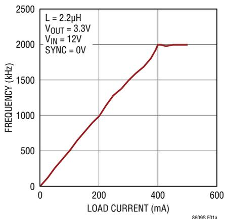
Figure 1a. SW Burst Mode Frequency vs Load
