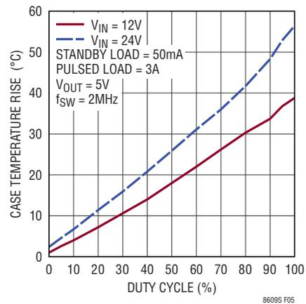
Figure 5. Case Temperature Rise vs 3A Pulsed Load
