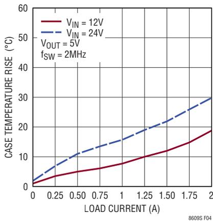
Figure 4. Case Temperature Rise vs Load Current
