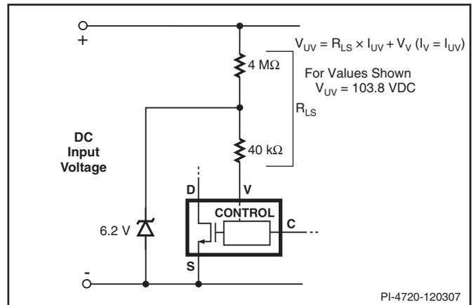
Figure 15. Line Sensing for Undervoltage Only (Overvoltage Disabled).
