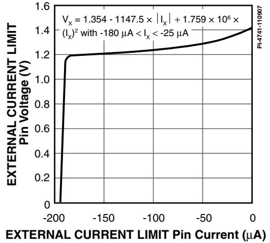
Figure 43. EXTERNAL CURRENT LIMIT Pin Voltage vs. Current.
