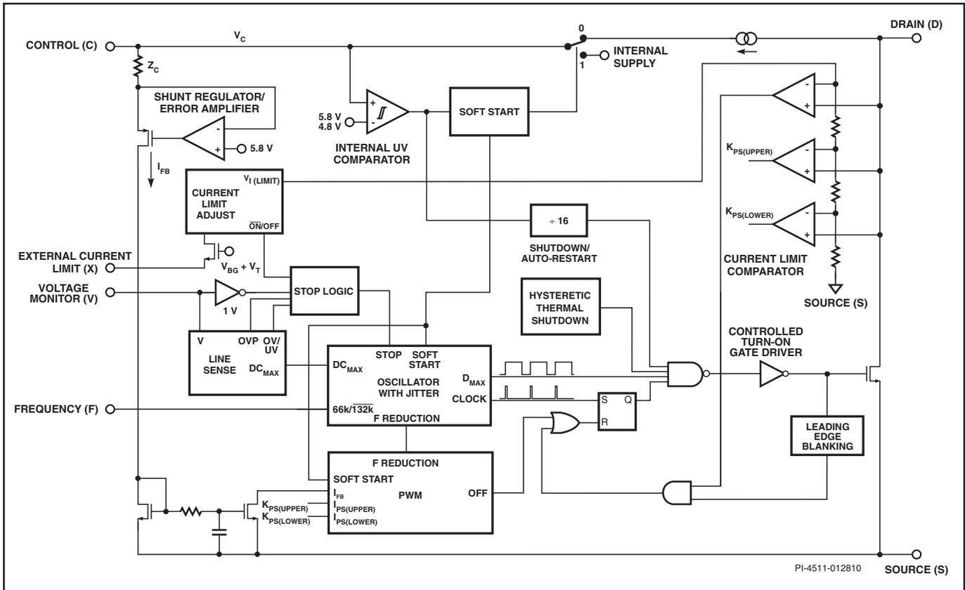
Figure 2. Functional Block Diagram (E and V Package).
