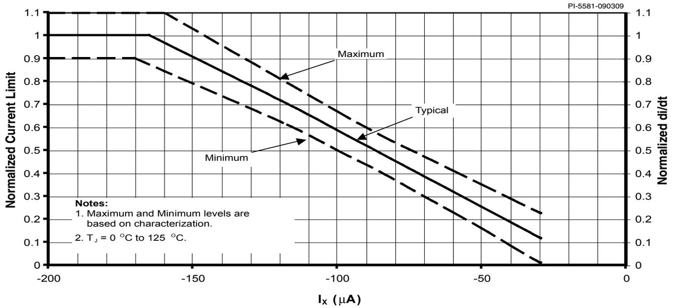
Figure 34. Normalized Current Limit vs. X Pin Current.
