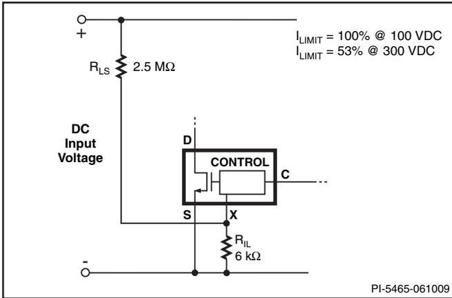
Figure 18. Current Limit Reduction with Line Voltage.
