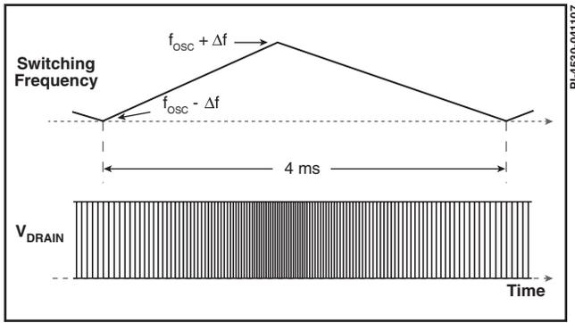
Figure 6. Switching Frequency Jitter (Idealized  $V_{DRAIN}$  Waveforms).
