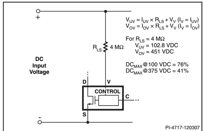
Figure 13. Line-Sensing for Undervoltage, Overvoltage and Line Feed-Forward.
