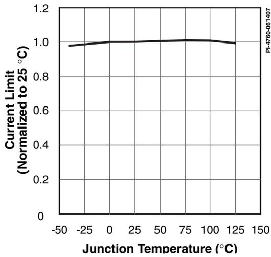
Figure 38. Internal Current Limit vs. Temperature.
