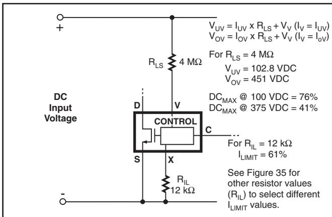
Figure 22. Line Sensing and Externally Set Current Limit.
