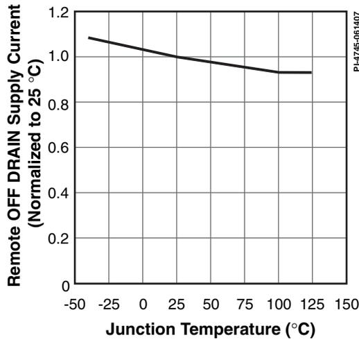
Figure 50. Remote OFF DRAIN Supply Current vs. Temperature.
