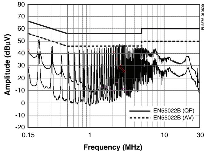
Figure 26. Fixed Frequency Operation Without Jitter.
