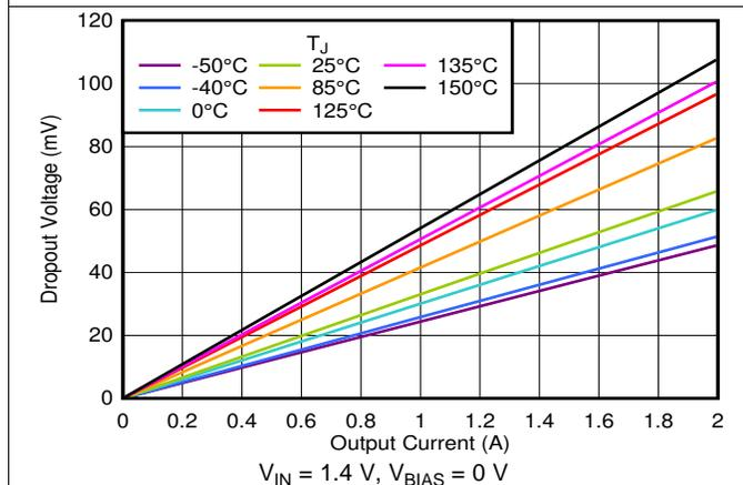
Figure 9. Dropout Voltage vs Output Current Without Bias
