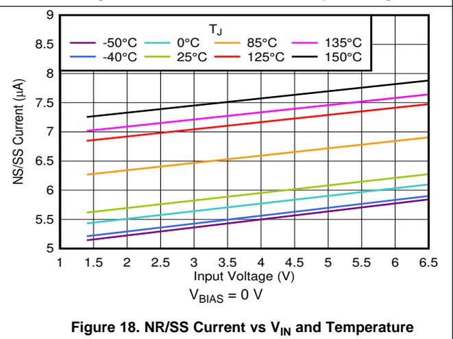
Figure 18. NR/SS Current vs  $V_{IN}$  and Temperature
