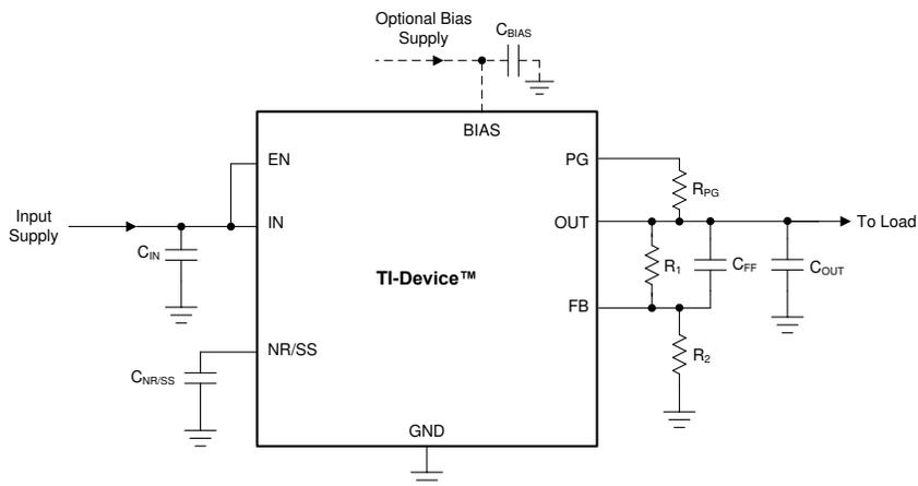
Figure 40. Typical Application for a 0.9-V Rail
