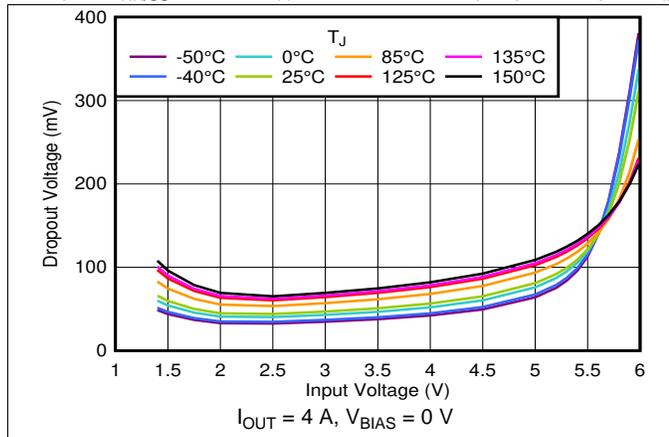
Figure 7. Dropout Voltage vs Input Voltage Without Bias
