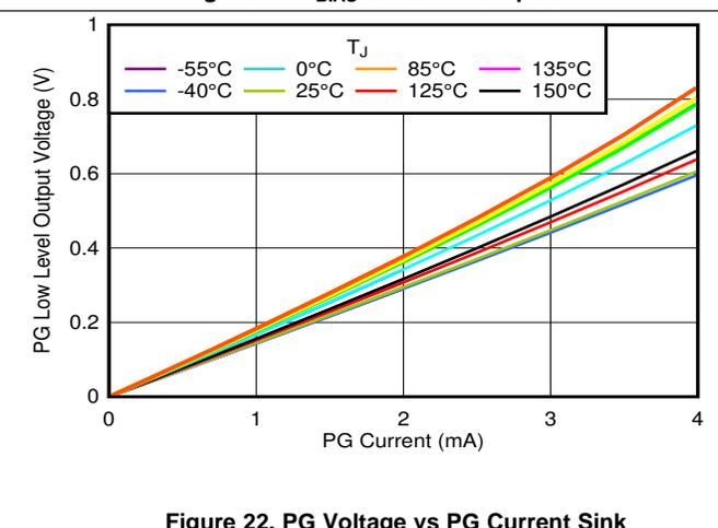
Figure 22. PG Voltage vs PG Current Sink
