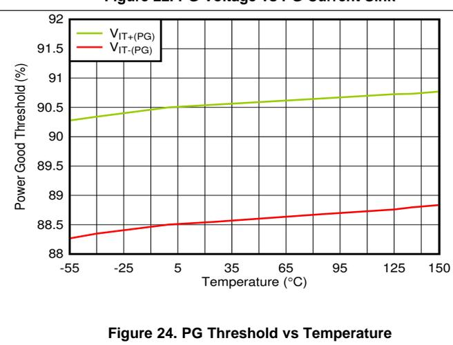
Figure 24. PG Threshold vs Temperature
