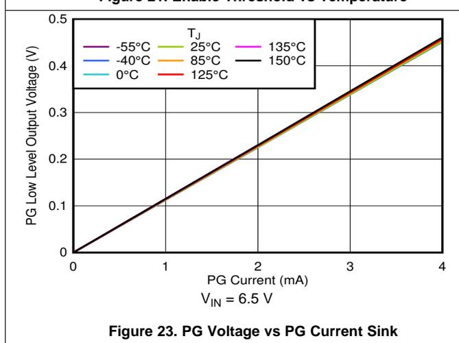
Figure 23. PG Voltage vs PG Current Sink
