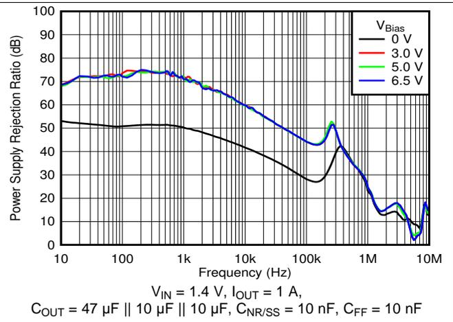
Figure 2. PSRR vs Frequency and  $V_{BIAS}$
