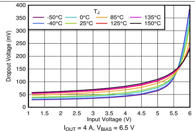
Figure 8. Dropout Voltage vs Input Voltage With Bias
