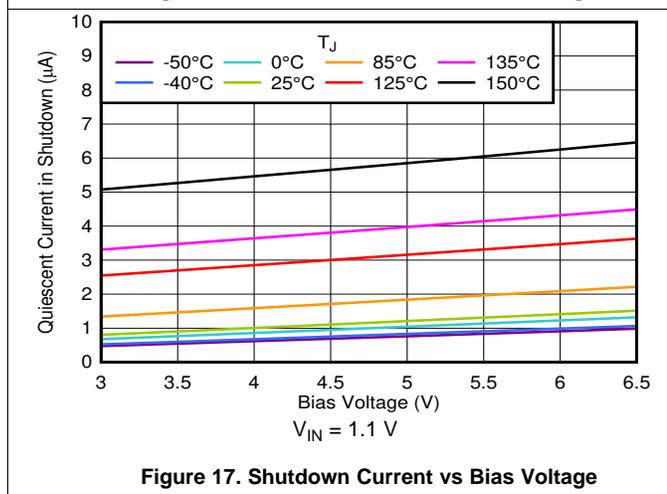
Figure 17. Shutdown Current vs Bias Voltage
