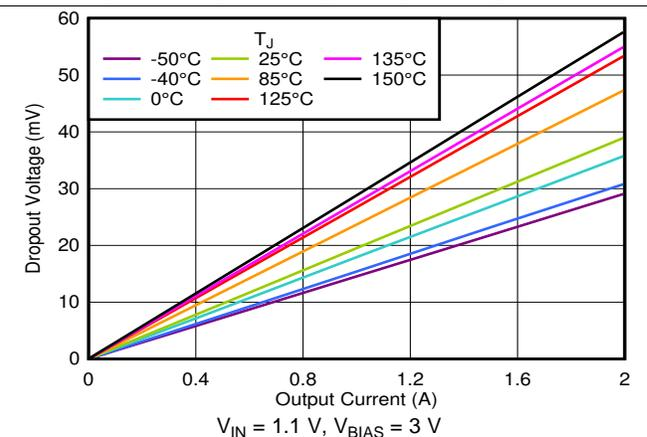
Figure 10. Dropout Voltage vs Output Current With Bias
