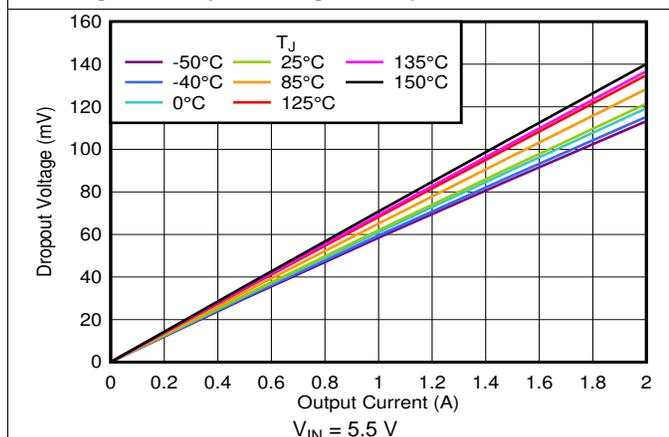
Figure 11. Dropout Voltage vs Output Current (High  $V_{IN}$ )
