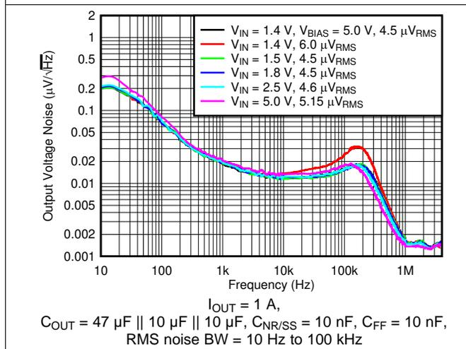
Figure 5. Output Voltage Noise vs Frequency and  $V_{IN}$
