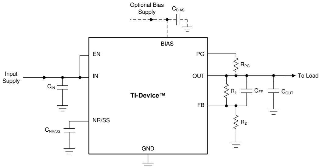
Figure 30. Adjustable Operation
