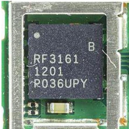
RF3161 (Quad band power amplifier module)
