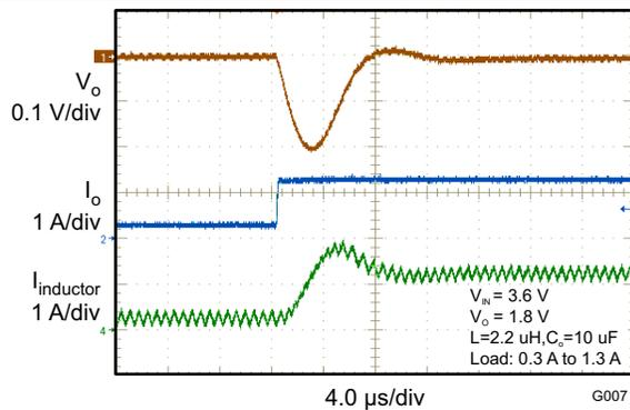
Figure 17. Load Transient
