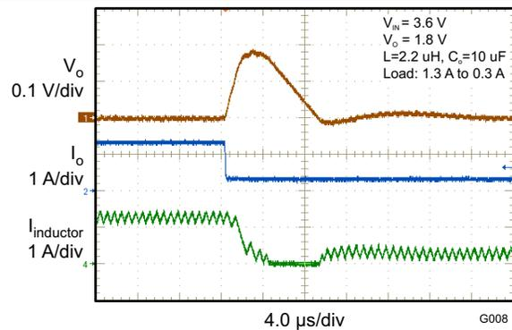
Figure 18. Load Transient
