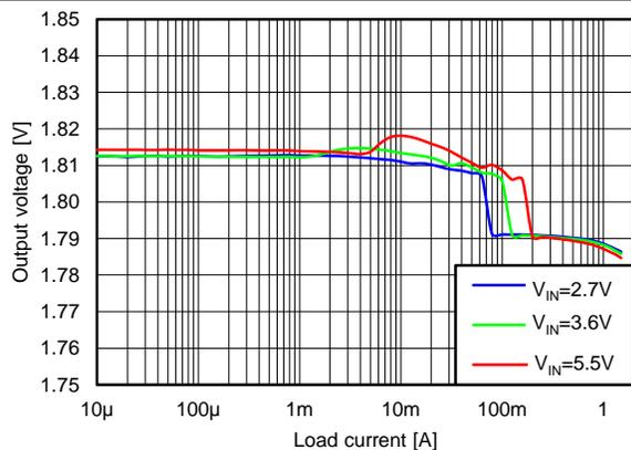
Figure 13. Output Voltage vs Load Current
