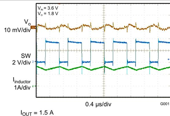
Figure 14. Typical Application (PWM Mode)
