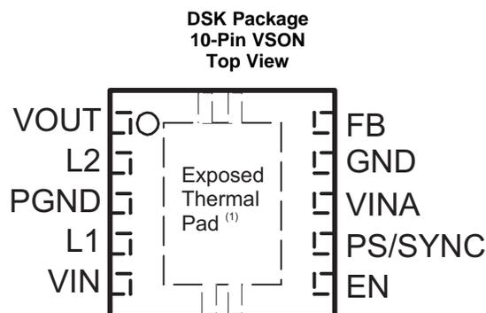
(1) The exposed thermal pad is connected to PGND.
