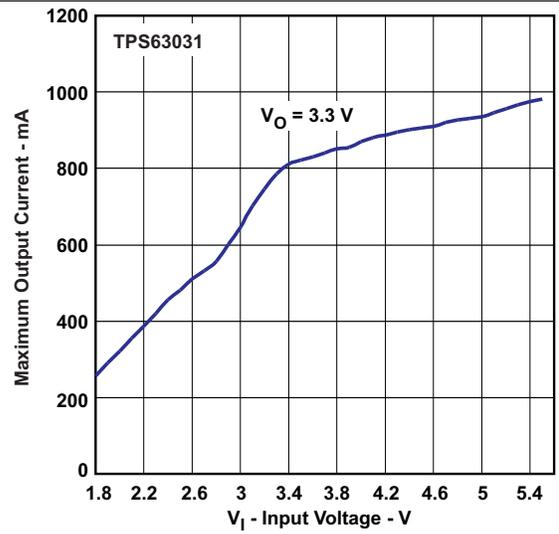
Figure 2. Maximum Output Current vs Input Voltage, TPS63031
