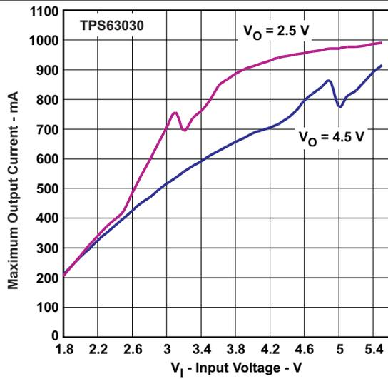
Figure 1. Maximum Output Current vs Input Voltage, TPS63030
