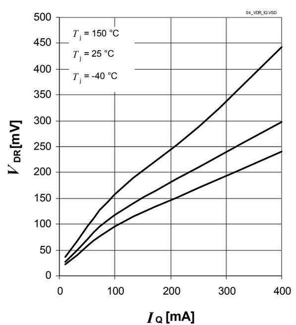
**Dropout Voltage  $V_{dr}$  versus Junction Temperature (5 V versions only)**
