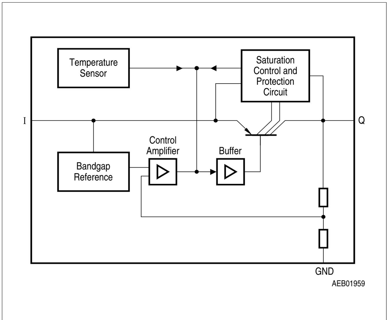
Figure 1 Block Diagram
