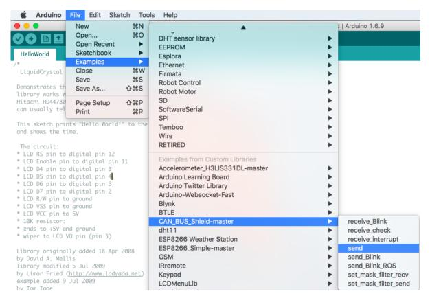
Open the receive\_check example (File > Examples > CAN\_BUS\_Shield-master >
