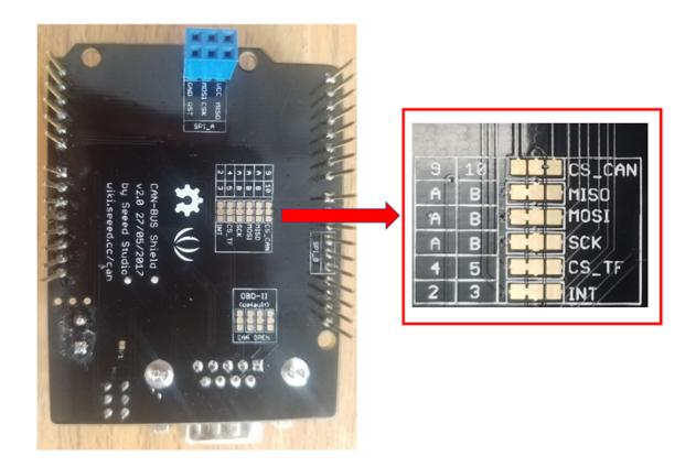
• Step2: Cut the wire between pad 2 and the middle pad.
