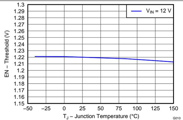
Figure 10. EN Pin Voltage vs Junction Temperature
