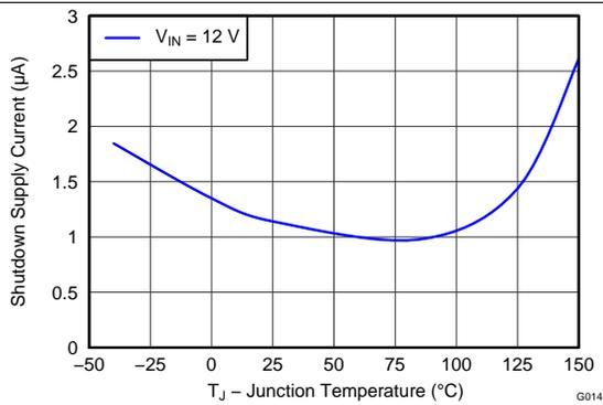
Figure 15. Shutdown Supply Current vs Junction Temperature
