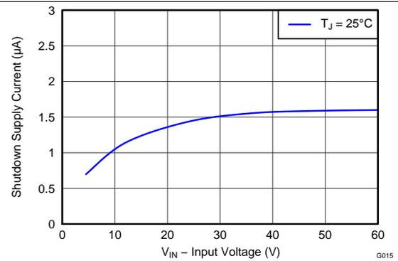
Figure 16. Shutdown Supply Current vs Input Voltage ( $V_{IN}$ )
