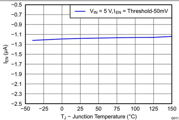
Figure 11. EN Pin Current vs Junction Temperature
