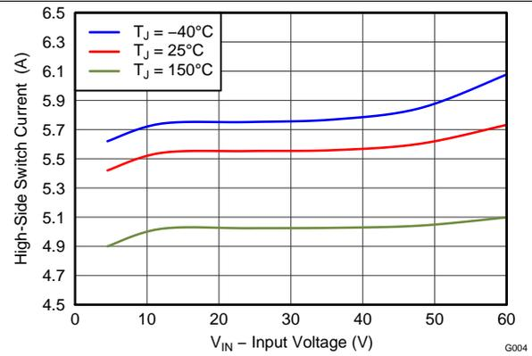
Figure 4. High-side Switch Current Limit vs Input Voltage
