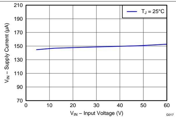
Figure 18.  $V_{IN}$  Supply Current vs Input Voltage
