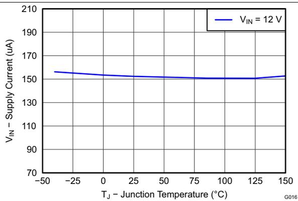
Figure 17.  $V_{IN}$  Supply Current vs Junction Temperature
