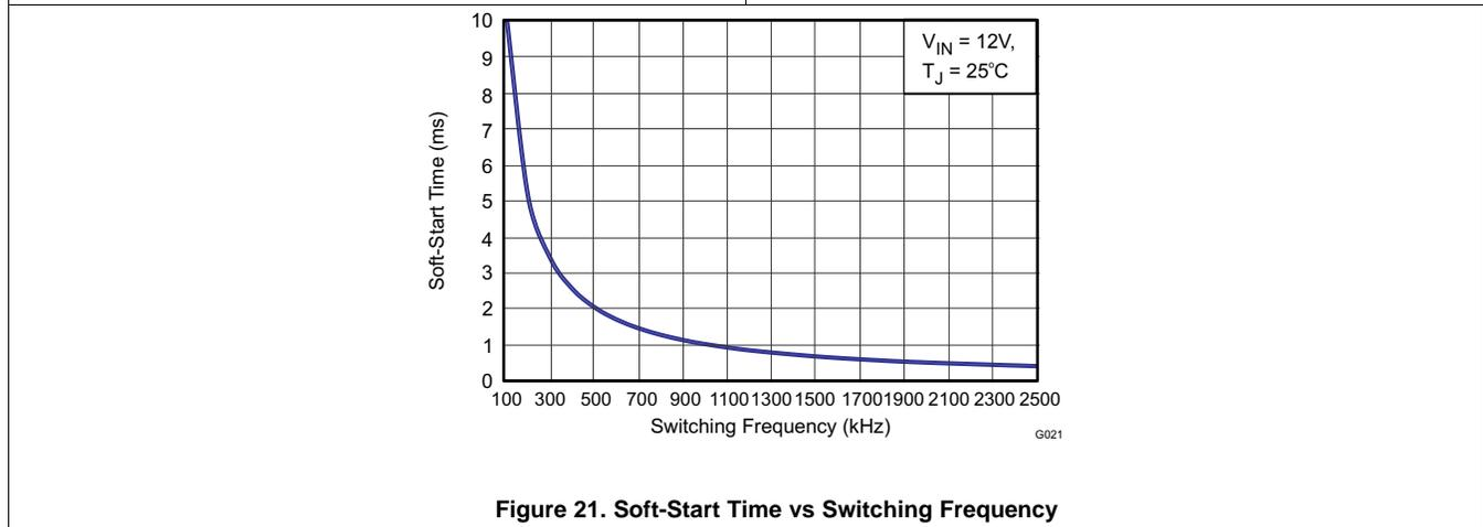
Figure 21. Soft-Start Time vs Switching Frequency
