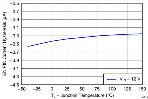
Figure 13. EN Pin Current Hysteresis vs Junction Temperature
