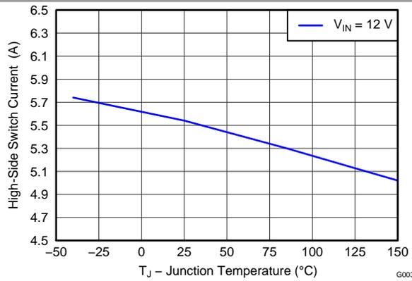
Figure 3. High-side Switch Current Limit vs Junction Temperature
