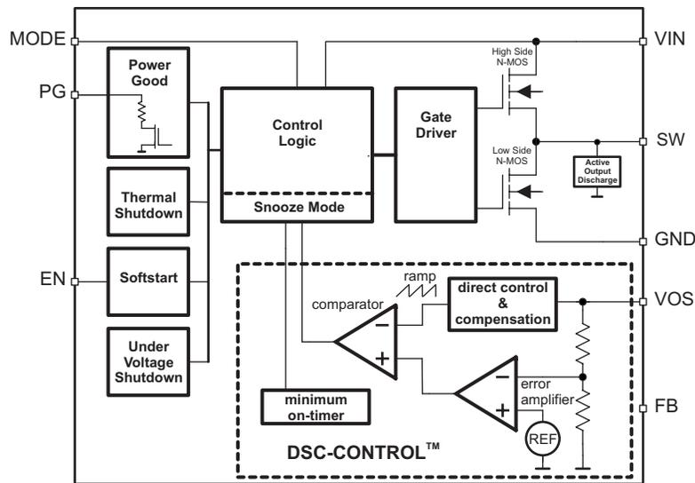
Figure 3. Functional Block Diagram (Fixed Output Voltage Version)
