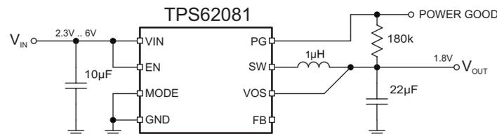
**Figure 1. Typical Application of TPS62081 (1.8V Fixed Output)**
