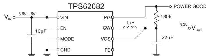
Figure 33. 3.3V Fixed Output Voltage Application (TPS62082)
