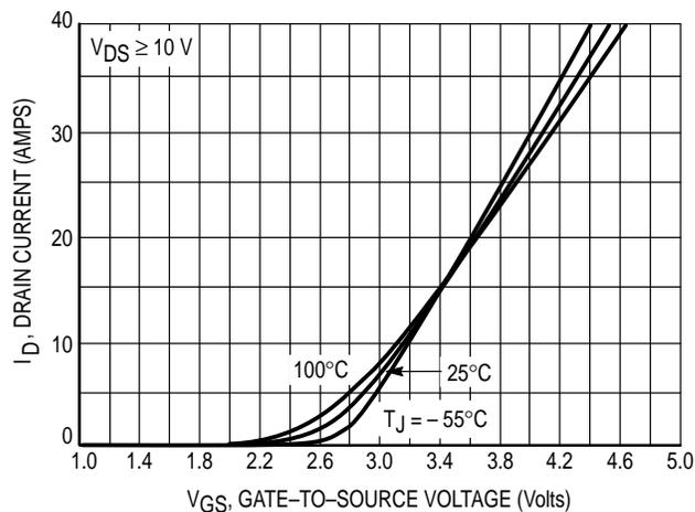
Figure 2. Transfer Characteristics
