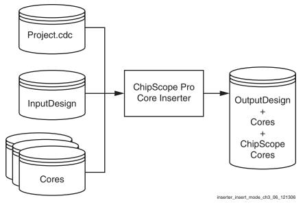
Figure 3-4: Insert Cores Step
