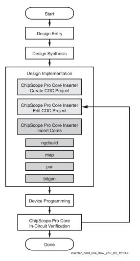
Figure 3-1: Command Line Core Inserter Flow
