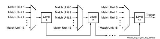
checkbox. A block diagram of the trigger sequencer is shown in Figure 3-5.
