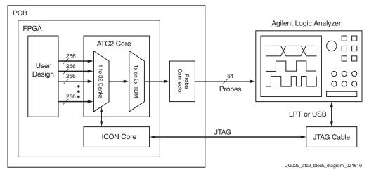
Figure 1-4: ATC2 Core and System Block Diagram
