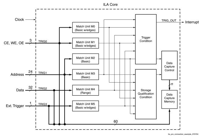
Figure 1-3: ILA Core Connection Example
