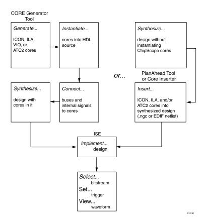
Figure 1-2: ChipScope Pro Tools Design Flow
