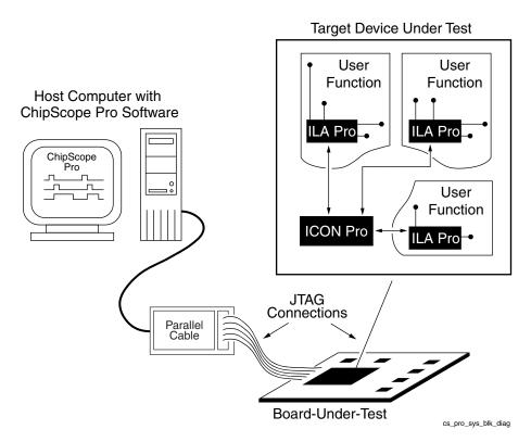
Figure 1-1: ChipScope Pro System Block Diagram
