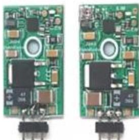
output voltage regulation modes: use fixed resistor or potentiometer (for ADJ)
