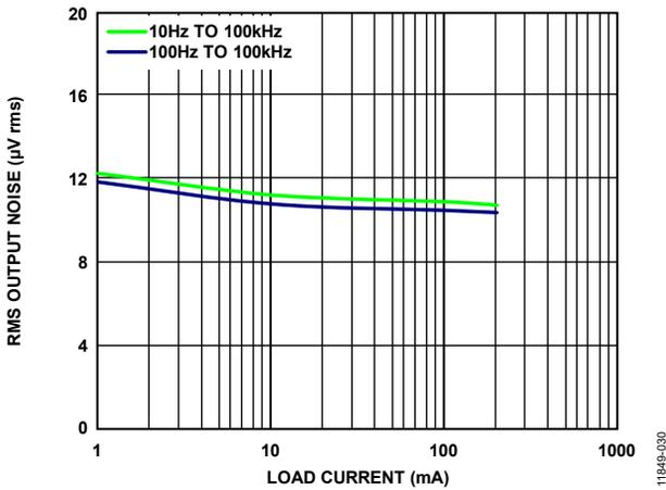
Figure 32. RMS Output Noise vs. Load Current
