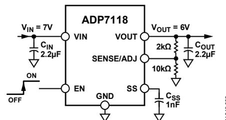
Figure 2. [ADP7118](#) with 5 V Output Adjusted to 6 V
