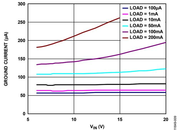
Figure 11. Ground Current vs. Input Voltage ( $V_{IN}$ )
