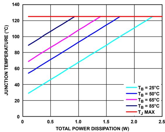
Figure 63. TSOT Junction Temperature Rise, Different Board Temperatures
