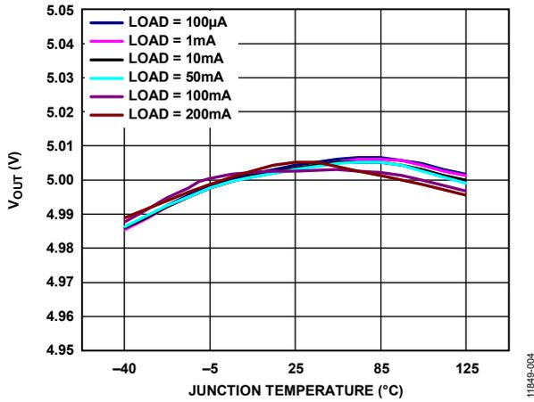
Figure 6. Output Voltage ( $V_{OUT}$ ) vs. Junction Temperature
