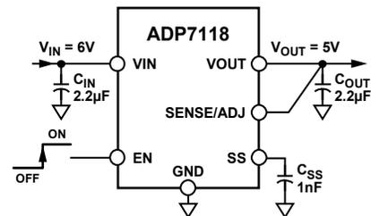
Figure 1. [ADP7118](#) with Fixed Output Voltage, 5 V
