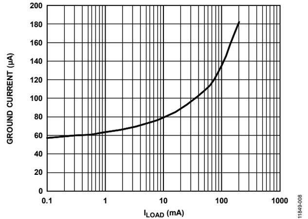
Figure 10. Ground Current vs. Load Current ( $I_{LOAD}$ )
