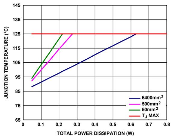
Figure 57. SOIC, T<sub>A</sub> = 85°C
