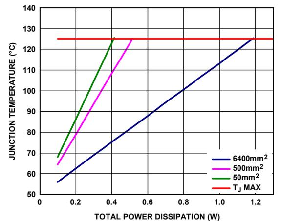
Figure 56. SOIC, T<sub>A</sub> = 50°C
