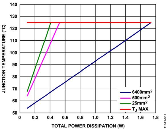
Figure 54. LFCSP, T<sub>A</sub> = 85°C
