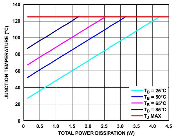
Figure 61. LFCSP Junction Temperature Rise, Different Board Temperatures
