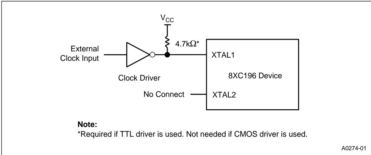
Figure 11. External Clock Connections
