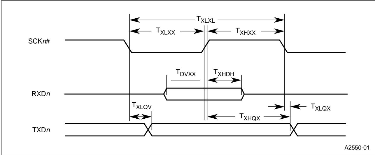
Figure 16. Serial Port Waveform — Mode 4
