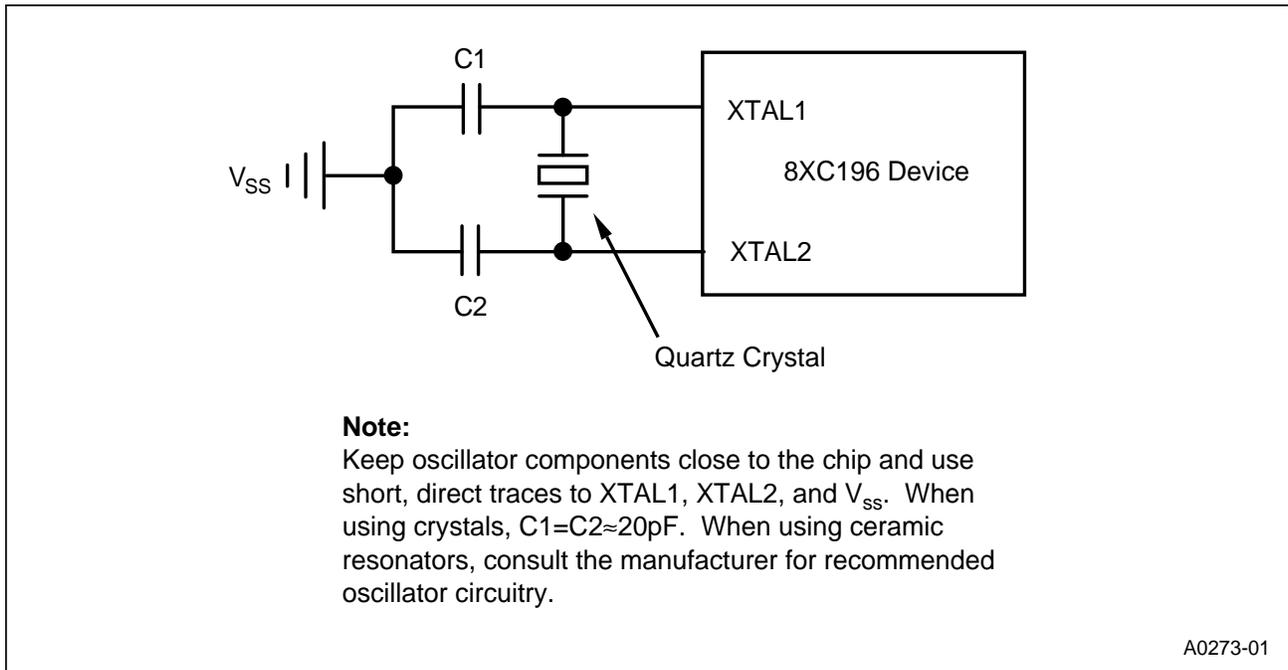
Figure 12. External Crystal Connections
