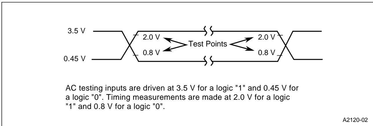
Figure 13. AC Testing Input, Output Waveforms
