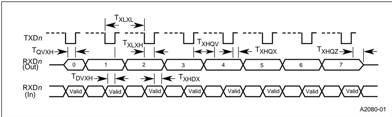
Figure 15. Serial Port Waveform — Shift Register Mode (Mode 0)
