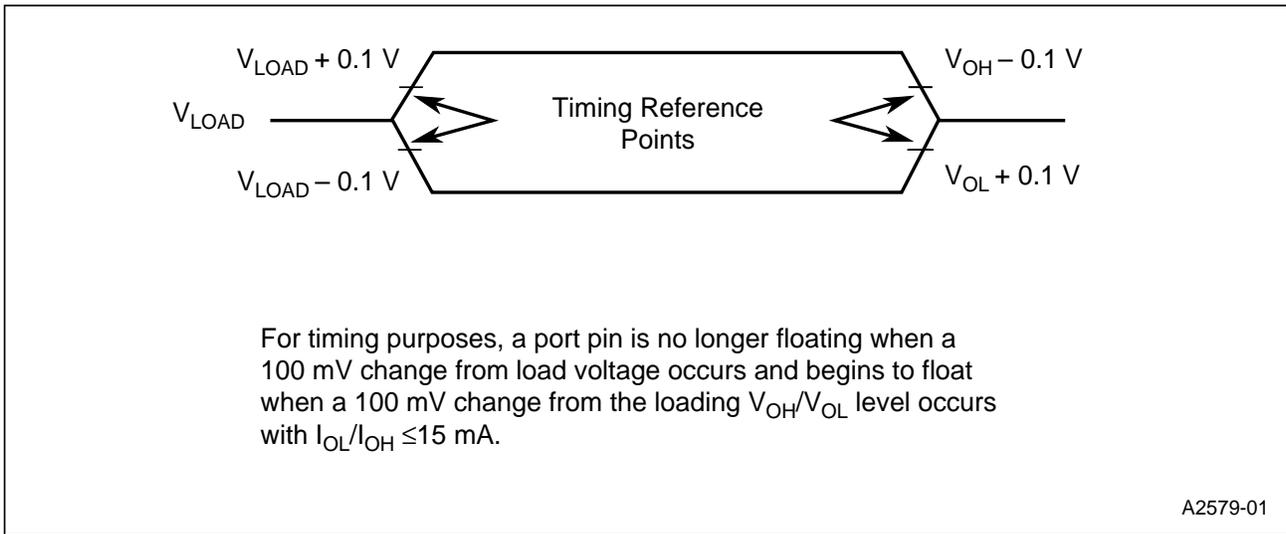
Figure 14. Float Waveforms
