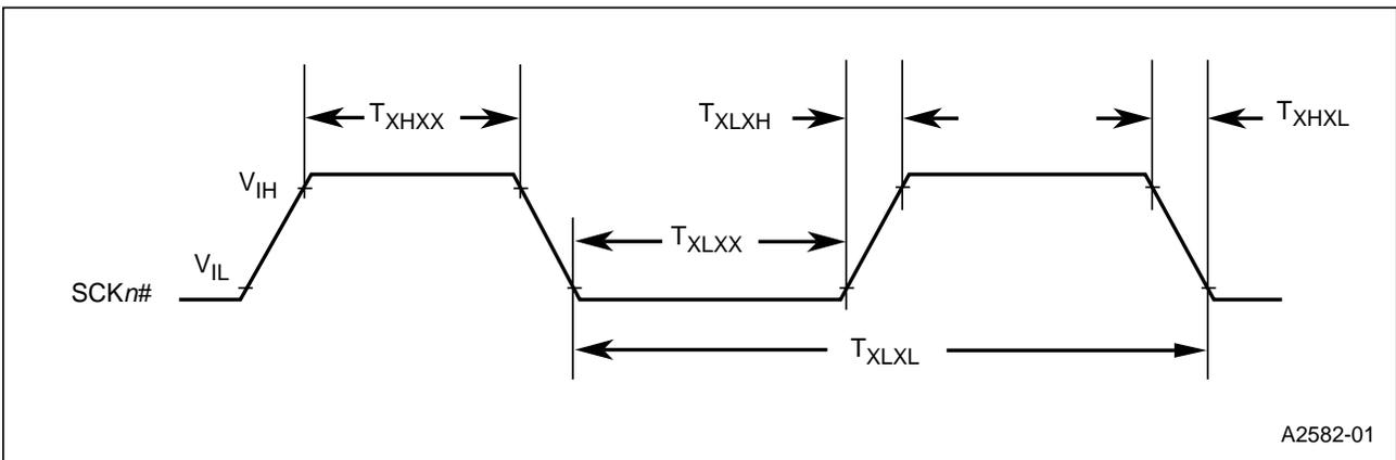
Figure 17. Serial Port Waveform — Clock Drive (DIR = 1)
