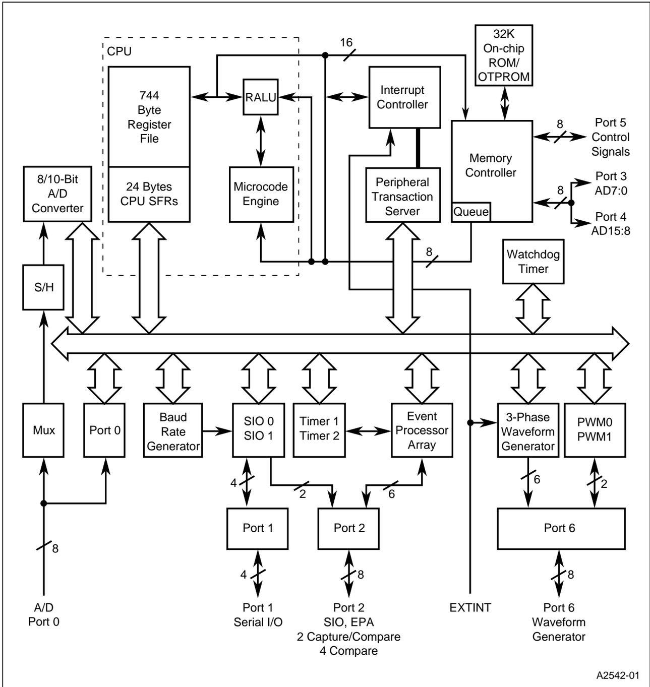
Figure 1. 8XC196MH Block Diagram
