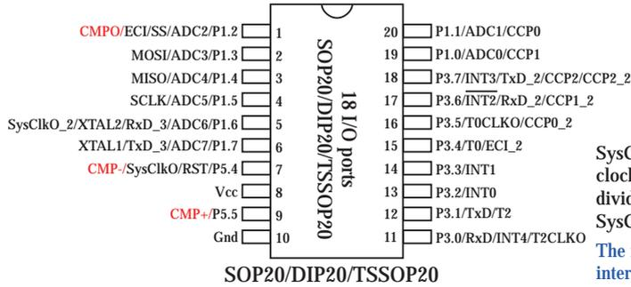
SysClk0 is the output of master clock whose frequency can be divided into SysClk/1, SysClk/2, SysClk/4
