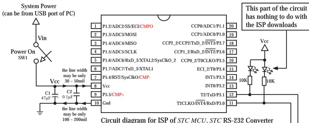
Please power on the target MCU after press down the button "Download/Program" on STC-ISP.exe when burning code to MCU.
