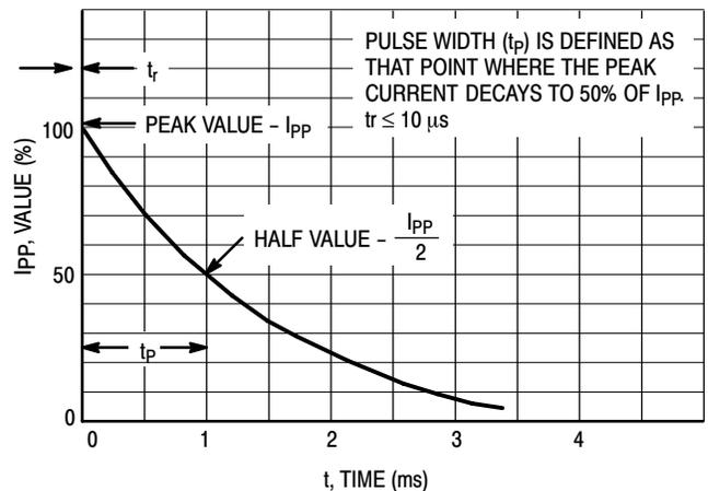
Figure 5. Pulse Waveform
