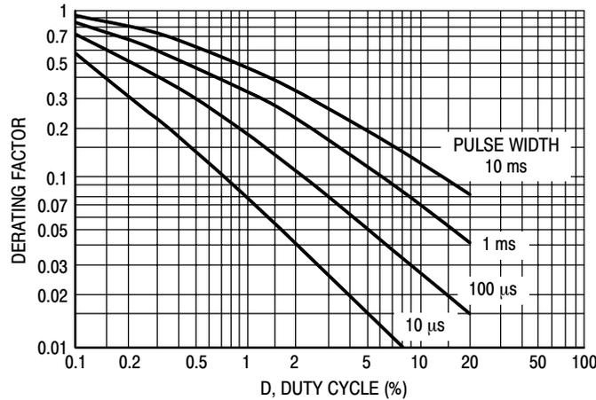
Figure 7. Typical Derating Factor for Duty Cycle
