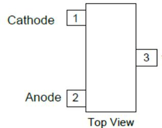
\* Pin 3 must be left floating or connected to pin 2
