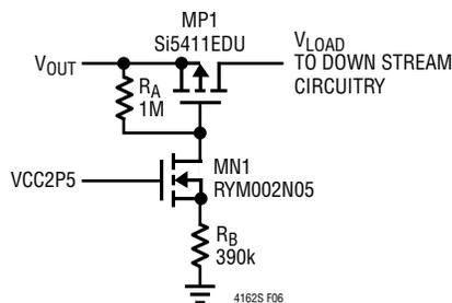
Figure 6. Isolating Downstream Circuits in Ship Mode.
