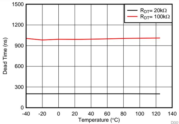
Figure 24. Dead Time vs. Temperature (with R<sub>DT</sub> = 20 kΩ and 100 kΩ)
