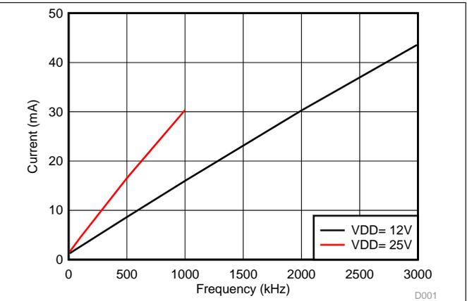
**Figure 5. Per Channel Current Consumption (I<sub>VDDA/B</sub>) vs. Frequency (1-nF Load, VDD = 12 V or 25 V)**
