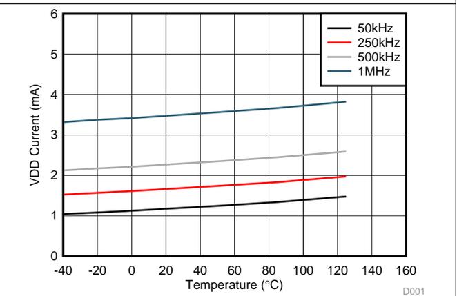
**Figure 7. Per Channel (I<sub>VDDA/B</sub>) Supply Current vs. Temperature (No Load, Different Switching Frequencies)**
