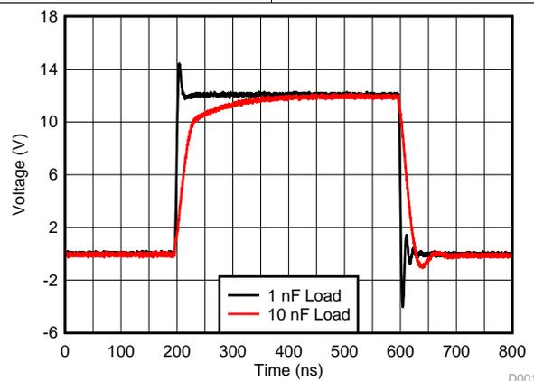
Figure 26. Typical Output Waveforms
