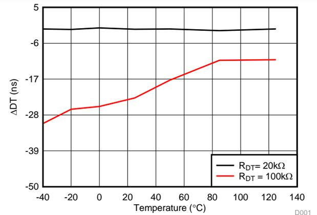
Figure 25. Dead Time Matching vs. Temperature (with R<sub>DT</sub> = 20 kΩ and 100 kΩ)
