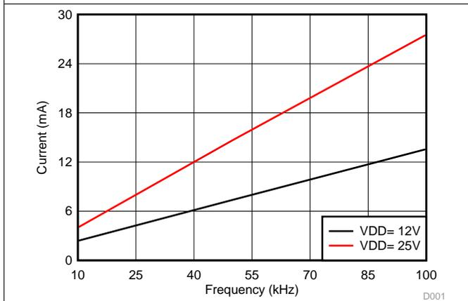
**Figure 6. Per Channel Current Consumption (I<sub>VDDA/B</sub>) vs. Frequency (10-nF Load, VDD = 12 V or 25 V)**
