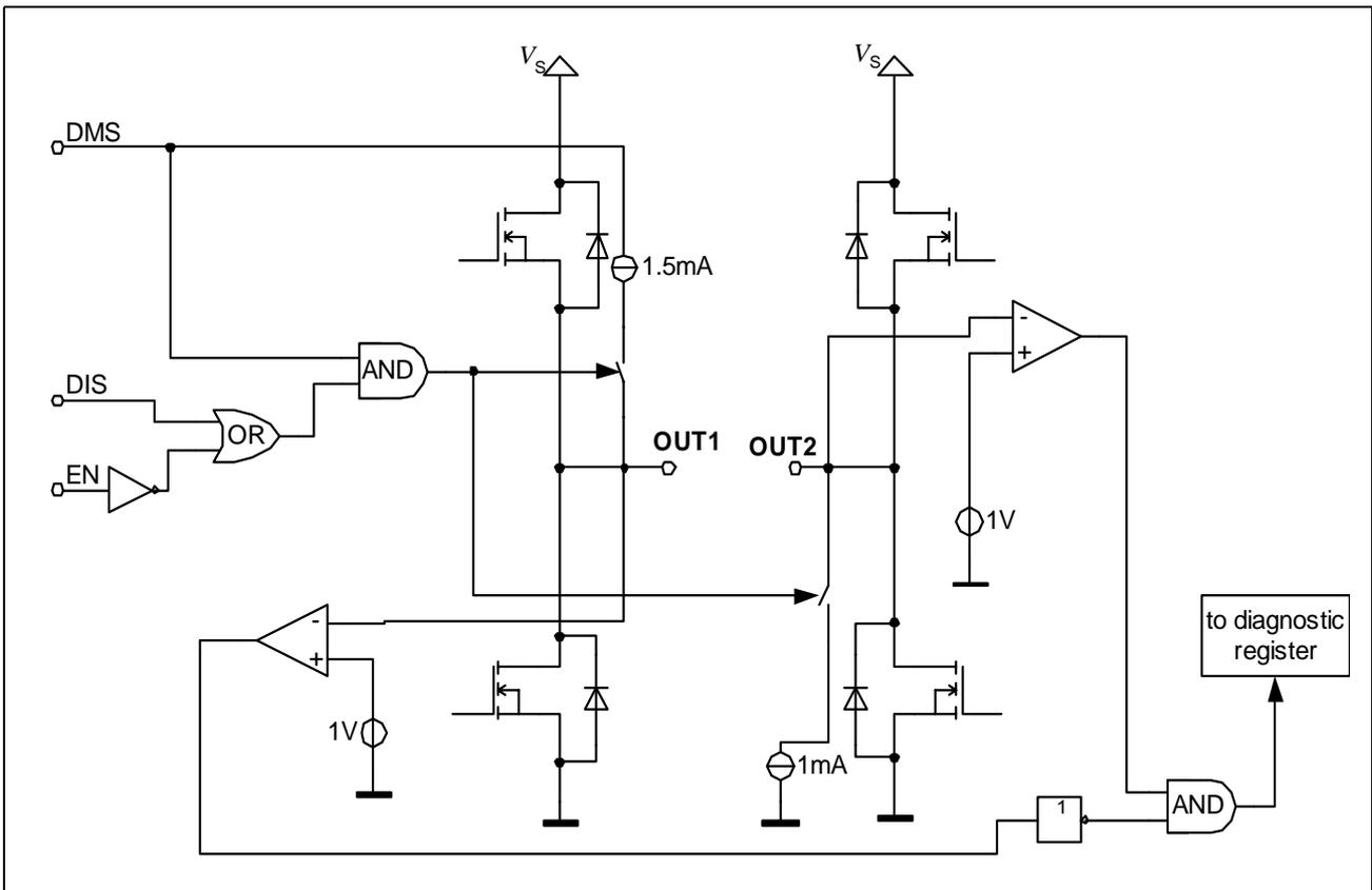
**Figure 9 Functional block diagram of open-load detection**
