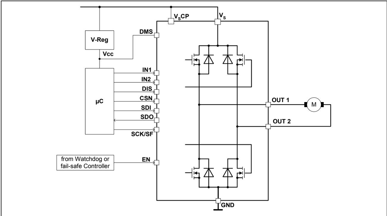
Figure 14 Application Example with SPI-Interface
