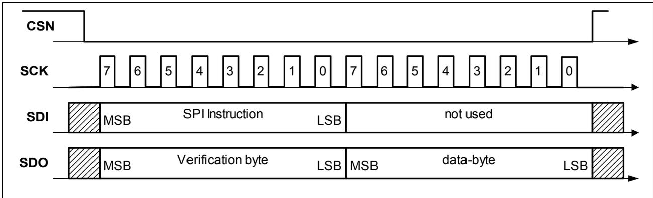
**Figure 8 SPI communication**
