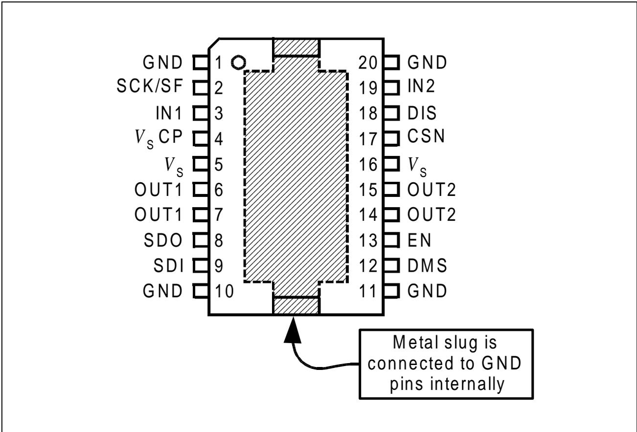
**Figure 1 Pinout TLE 7209-2R**
