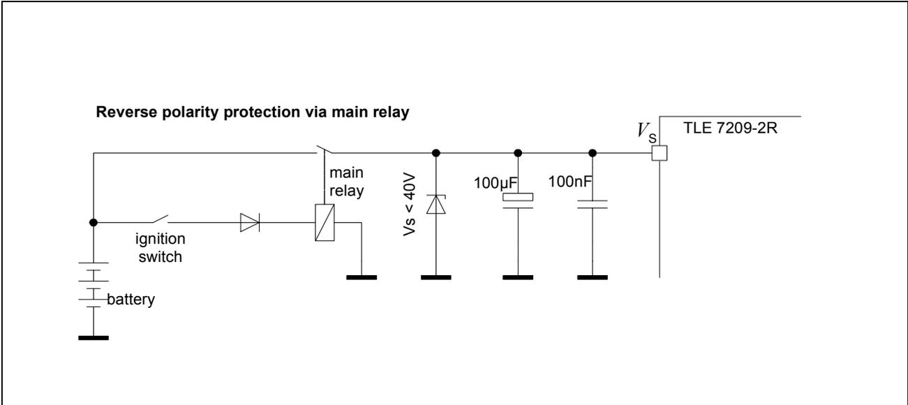
**Figure 16 Application Examples for Over-Voltage- and Reverse-Voltage Protection**
