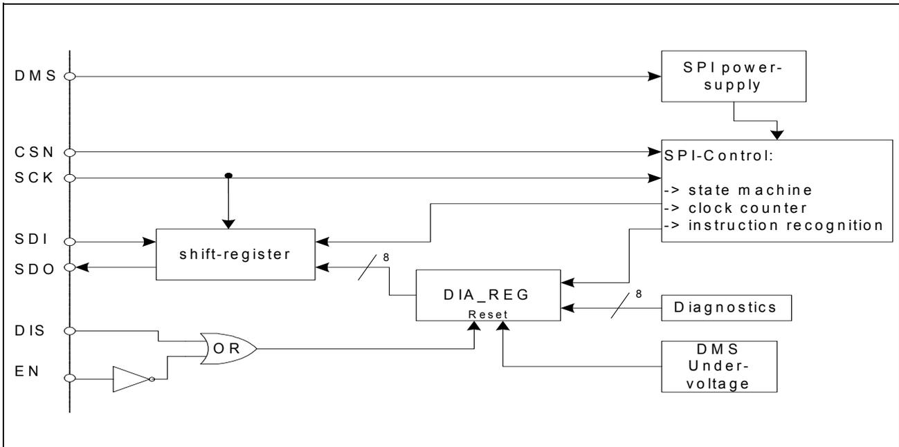
**Figure 6 SPI block-diagram**
