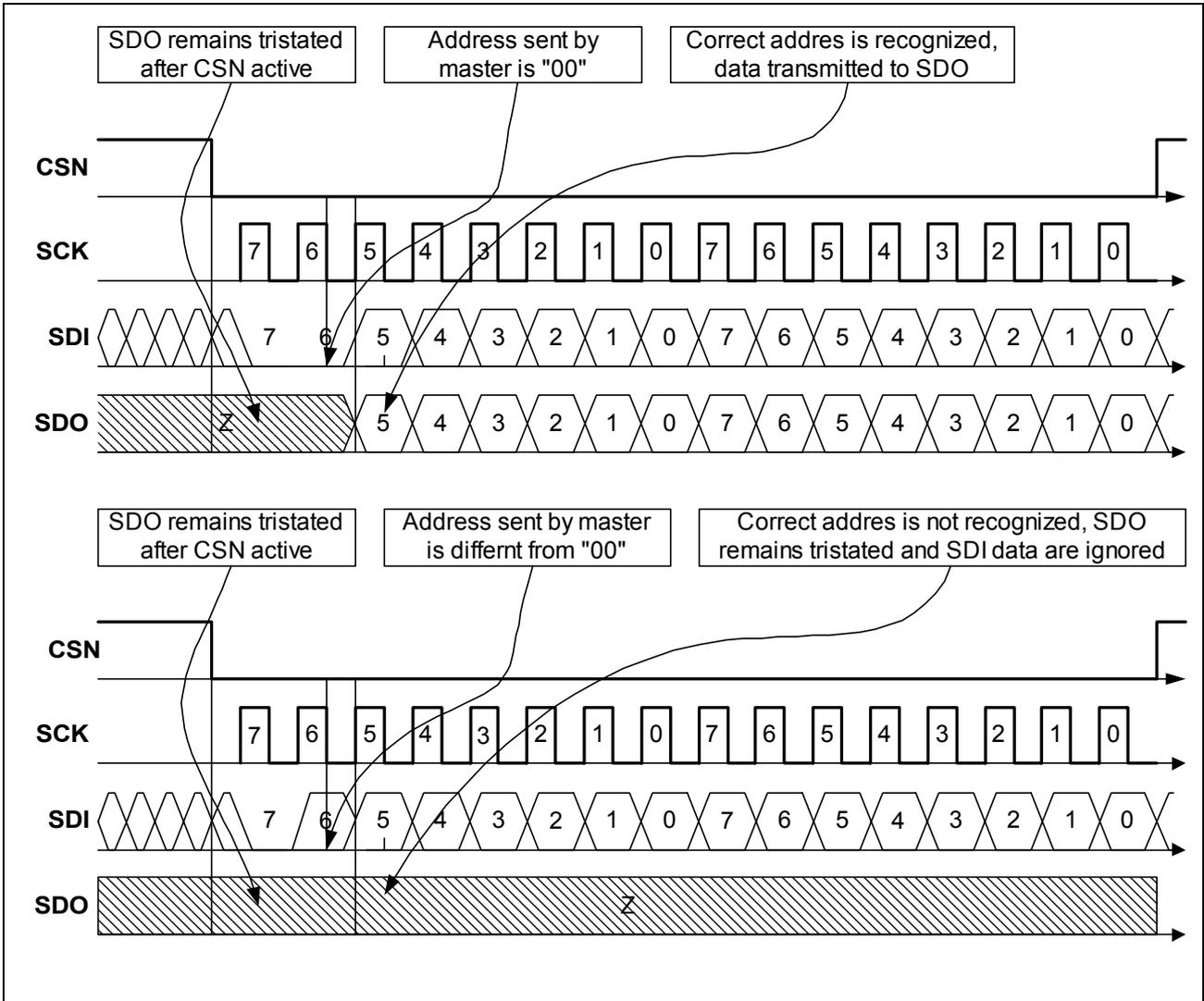
Figure 7 Bus-arbitration by chip-address
