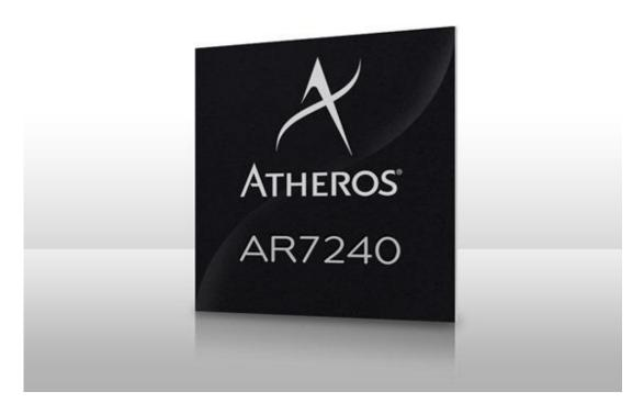
The AR7240 includes a MIPS 24K core processor, a PCI-e Host host device interface, an integrated 5-port 100M Ethernet switch (MAC / PHY), a USB 1.1 MAC / PHY, and an SPI. External memory interface, DDR1 / DDR2 interface, a high-speed UART interface, and some GPIO.
