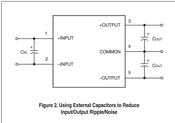
Figure 2. Using External Capacitors to Reduce Input/Output Ripple/Noise
