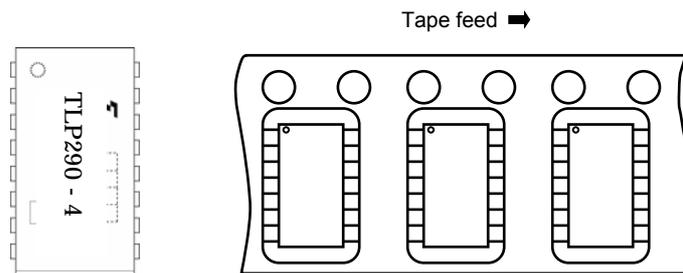
**Figure 1 Device Orientation**
