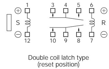
S : Coil polarity of set (operate)
