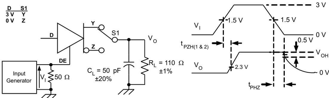
Generator: PRR = 500kHz, 50% Duty Cycle,  $t_r < 6 \text{ ns}$ ,  $t_f < 6 \text{ ns}$ ,  $Z_o = 50 \Omega$
