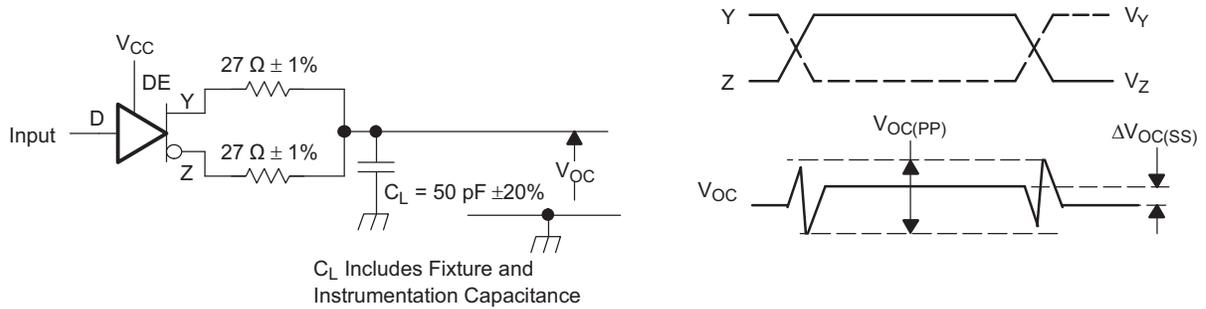
Input: PRR = 500 kHz, 50% Duty Cycle,  $t_r < 6ns$ ,  $t_f < 6ns$ ,  $Z_0 = 50 \Omega$
