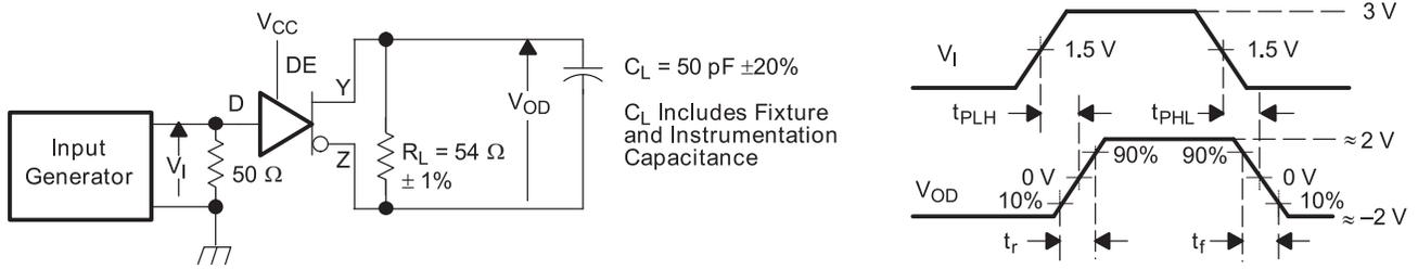
Generator: PRR = 500 kHz, 50% Duty Cycle,  $t_r < 6 \text{ ns}$ ,  $t_f < 6 \text{ ns}$ ,  $Z_o = 50 \Omega$
