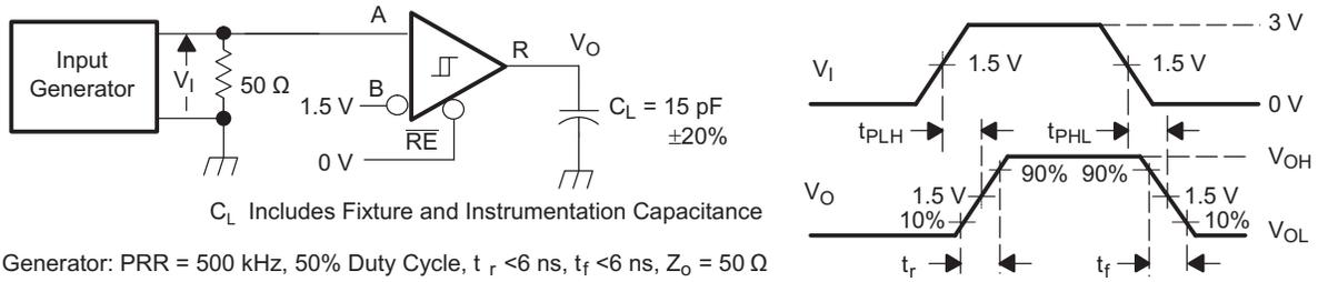
Figure 9. Receiver Switching Test Circuit and Voltage Waveforms
