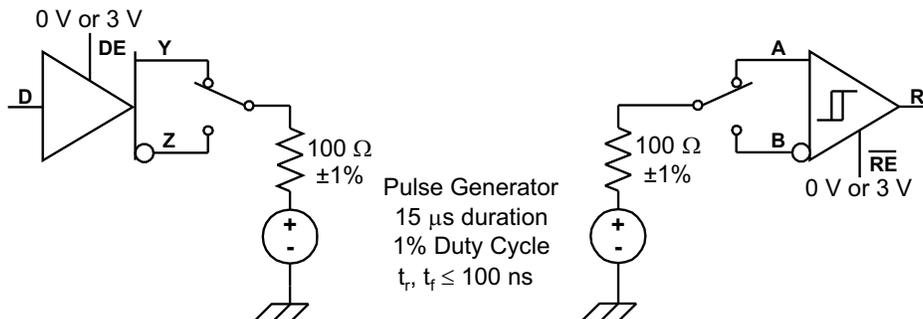
Figure 12. Test Circuit, Transient Over Voltage Test
