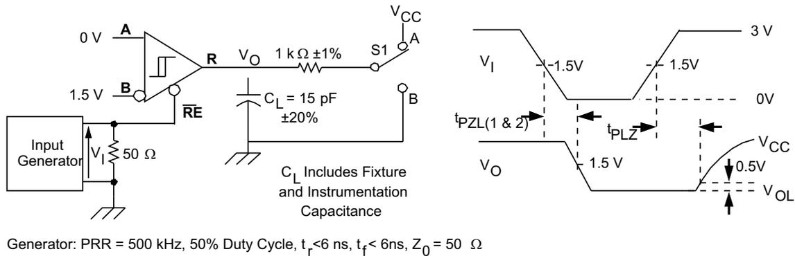
Figure 11. Receiver Enable Time From Standby (Driver Disabled)
