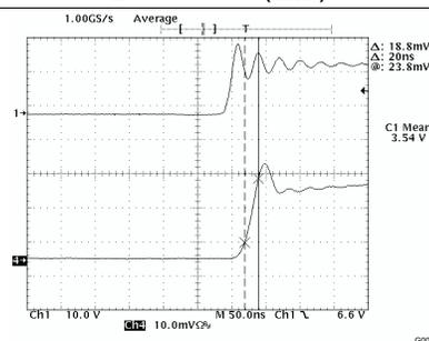
Figure 6. Input Current With Slope Control, SCR0 = 1, SCR1 = 1, Input-Current Slew Rate =  $18.8 \text{ A}/\mu\text{s}$ ,  $I_L = 500 \text{ mA}$ ,  $V_{(driver)} = 15 \text{ V}$
