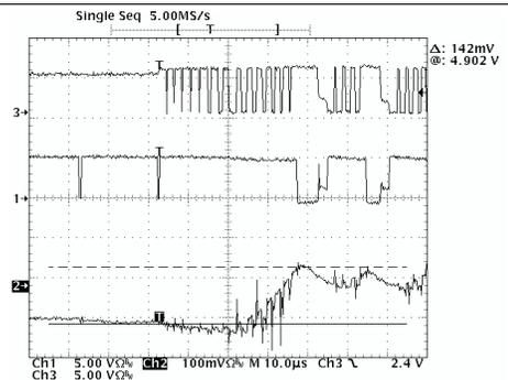
Figure 12. Switched-Mode Regulator Transition from Buck Mode to Boost Mode,  $I_L = 400 \text{ mA}$
