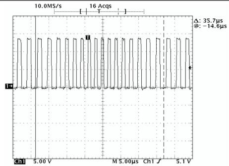
Figure 10. Modulation Frequency (Full Span) of 28 kHz
