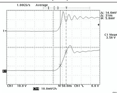
Figure 5. Input Current with Slope Control, SCR1 = 1, SCR0 = 0, Input-Current Slew Rate =  $9.4 \text{ A}/\mu\text{s}$ ,  $I_L = 500 \text{ mA}$ ,  $V_{(driver)} = 15 \text{ V}$
