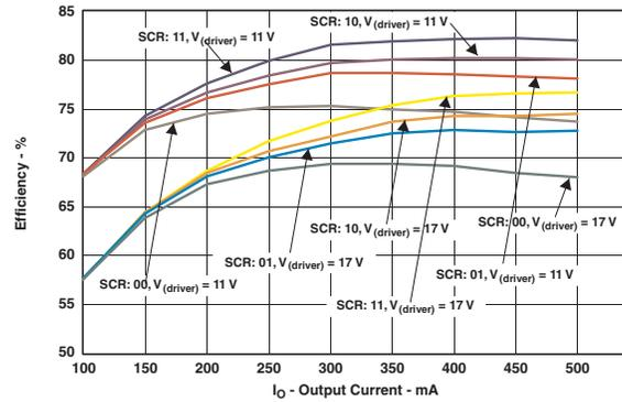
Figure 20. Converter Efficiency
