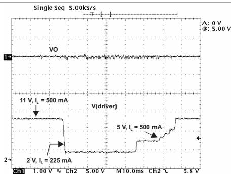
Figure 11. Input Voltage Excursions (Similar to Low-Crank Conditions)
