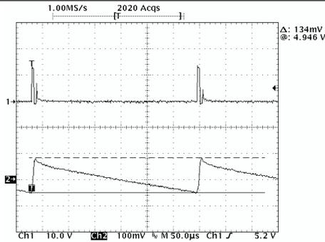
Figure 7. Low-Power-Mode Operation,  $I_L = 15 \text{ mA}$ ,  $C_O = 47 \mu\text{F}$
