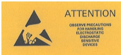
Although quartz is not necessarily susceptible to ESD damage, the associated electronic circuitry contained within an oscillator *is* and should be considered as an Electrostatic Discharge Sensitive device (ESDS).
