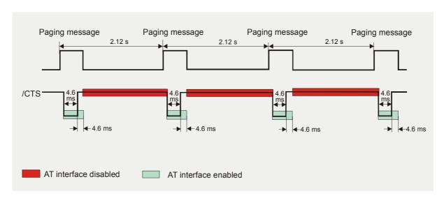
Figure 8: Timing of /CTS signal (example for a 2.12 s paging cycle)
