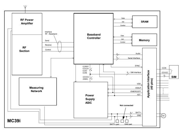
Figure 1: Block diagram of MC39i
