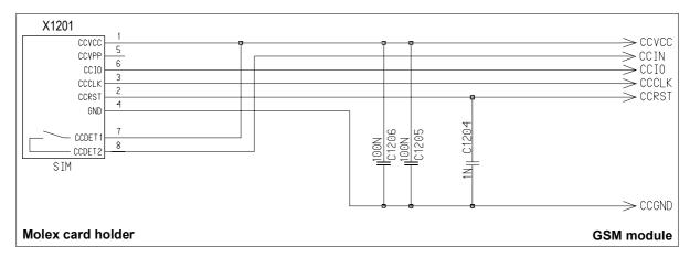
Figure 13: SIM card holder of DSB35 Support Box
