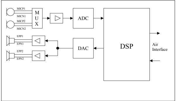
Figure 12: Audio block diagram
