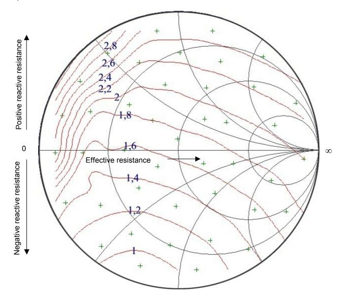
Figure 25: Peak current during transmit burst in A vs. antenna impedance
