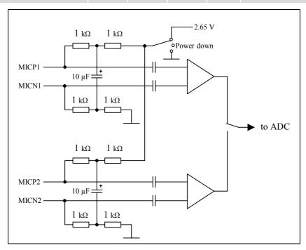
Figure 27: Structure of audio inputs
