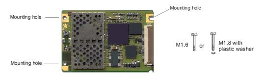
Figure 30: Recommended screws
