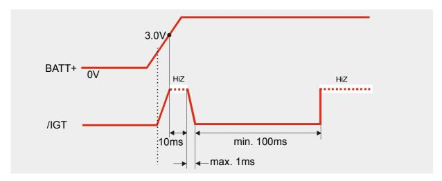
Figure 5: Timing of power-on process if VDDLP is not used
