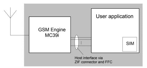
Figure 2: Block diagram of a cellular application
