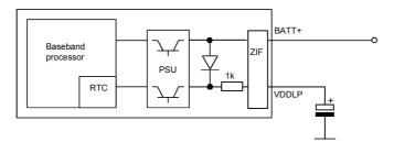
Figure 10: RTC supply from capacitor
