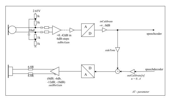
Figure 26: AT audio programming model
