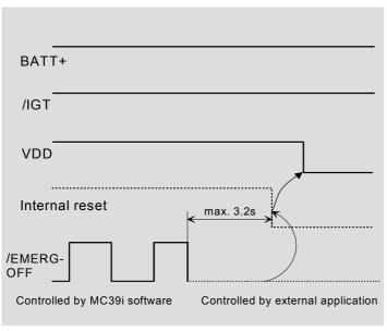
Figure 7: Deactivating GSM engine by Power Down signal
