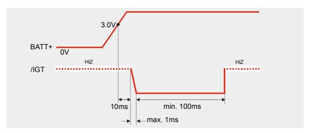
Figure 6: Timing of power-on process if VDDLP is fed from external source
