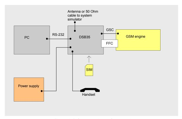
Figure 33: Reference equipment for approval
