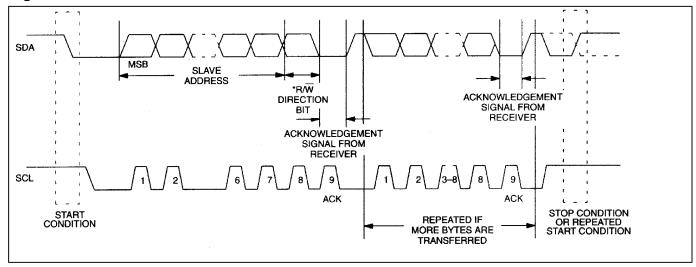
Figure 3. Data Transfer on I<sup>2</sup>C Serial Bus
