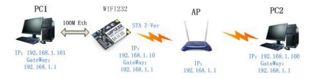
Figure 22 WIFI232 Ethernet Interface Networking (As STA, Z-Ver)
