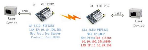
Figure 51 Configure Transparent Serial Port Connection (TCP)
