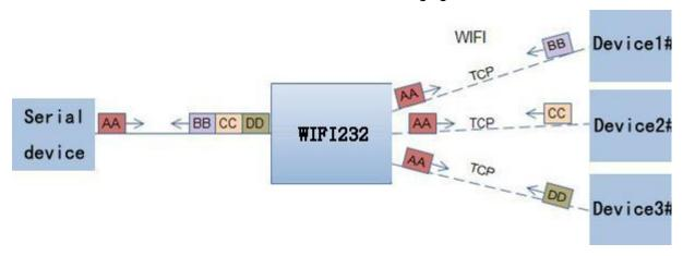
Figure 24 Multi-TCP Link Data Transmition Structure
