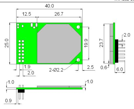
Figure 9 WIFI232 Mechanical Size
