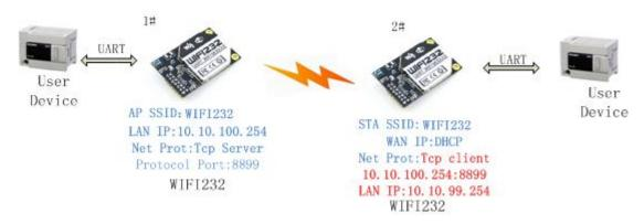
Figure 49 Transparent Serial Port Application
