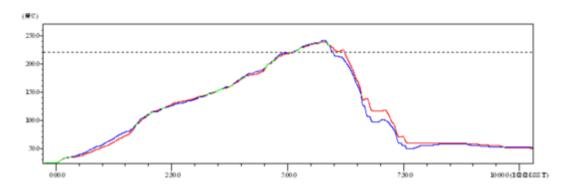
Figure 5 Reflow Soldering Profile
