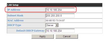
Figure 52 Module LAN IP Setting
