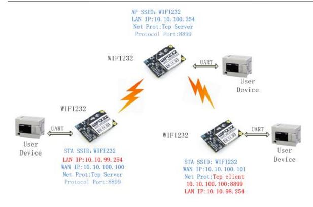
Figure 58 Two WIFI232 Modules Connection Through AP
