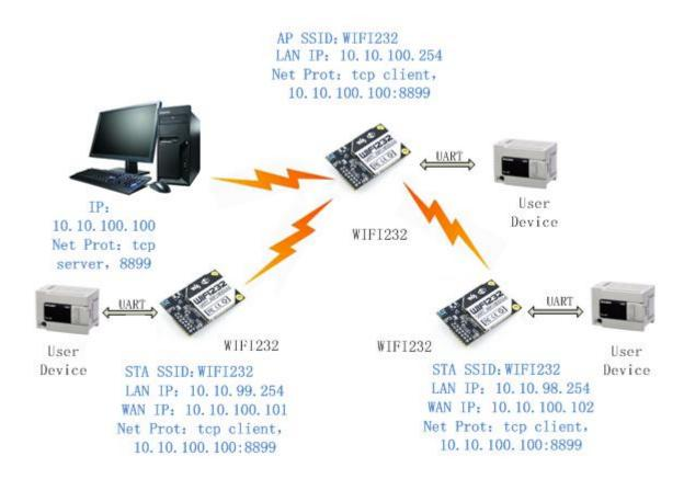
Figure 59 Wireless Data Acquisition Card Setting
