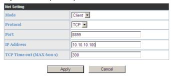
Figure 56 Module Network Protocol: TCP/Client
