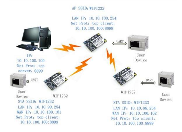
Figure 50 Wireless Data Acquisition Card Application
