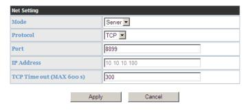
Figure 55 Module Network Protocols: TCP/Server
