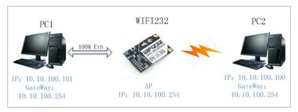
Figure 20 WIFI232 Ethernet Interface Networking (As AP)
