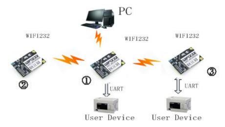
Figure 18 WIFI232 STA Network Structure
