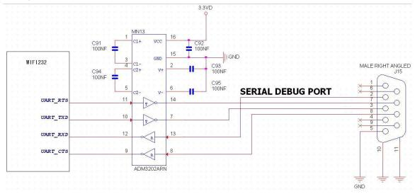
Figure 15 Figure 1 UART Interface Reference Design
