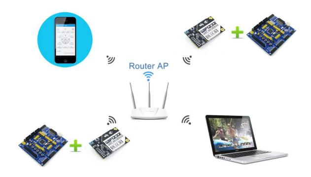
Figure 17 WIFI232 Basic Wireless Network Structure
