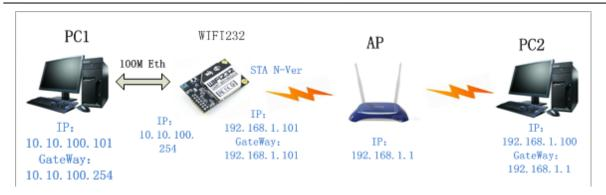
Figure 21 WIFI232 Ethernet Interface Networking (As STA, N-Ver)
