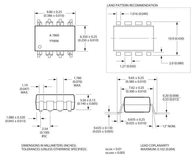
NOTE: FLOATING LEAD PROTRUSION IS 0.5 mm (20 mils) MAX.
