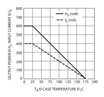
b. See Figure 1 for dependence of PS and IS on ambient temperature.
