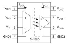
NOTE: A 0.1-µF bypass capacitor must be connected between pins 1 and 4 and between pins 5 and 8.
