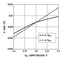
Figure 9: Nonlinearity vs. Supply
