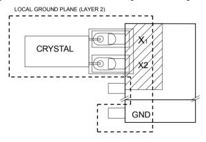
NOTE: AVOID ROUTING SIGNAL LINES IN THE CROSSHATCHED AREA (UPPER LEFT QUADRANT) OF THE PACKAGE UNLESS THERE IS A GROUND PLANE BETWEEN THE SIGNAL LINE AND THE DEVICE PACKAGE.
