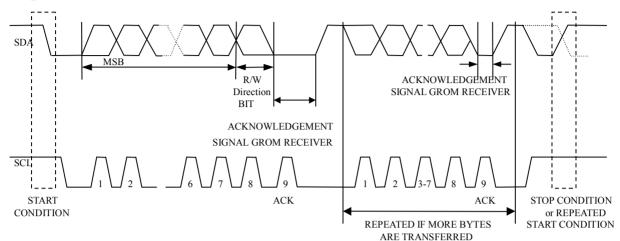
Figure 4. Data Transfer on I<sup>2</sup>C Serial Bus
