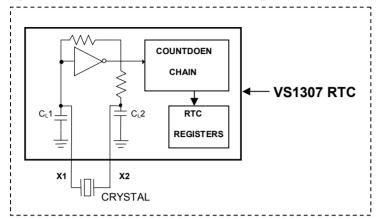
Figure 3 Oscillator Circuit Showing Internal Bias Network
