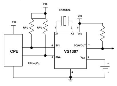
Figure 1. Block Diagram
