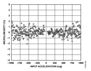
Figure 9. X-Axis Microlinearity, 50 mg Step Size
