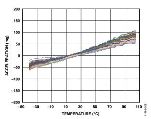
Figure 5. Z-Axis Acceleration vs. Temperature, Three Lots (N = 80)
