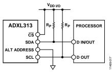
Figure 20. I<sup>2</sup>C Connection Diagram (Address 0x53)
