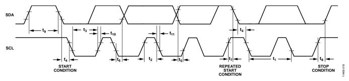
Figure 22. I<sup>2</sup>C Timing Diagram
