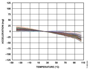
Figure 4. Y-Axis Acceleration vs. Temperature, Three Lots (N = 80)
