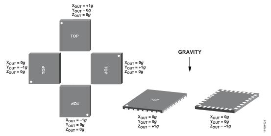
Figure 28. Output Response vs. Orientation to Gravity
