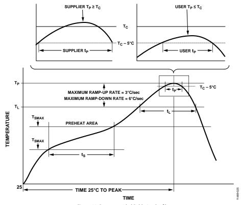
Figure 29. Recommended Soldering Profile
