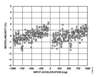
Figure 11. Z-Axis Microlinearity, 50 mg Step Size
