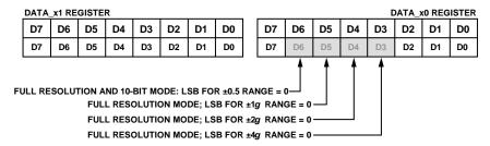
FOR THE LEFT JUSTIFIED DATA: WHEN OPERATING THE ADXL313 WITH AN OUTPUT RATE OF EITHER 3200Hz OR 1600Hz, THE LSB OF THE ACCELERATION DATA-WORD IS ALWAYS 0 UNDER THE FOLLOWING CONDITIONS: 1) FULL RESOLUTION MODE IS ENABLED (ANY g RANGE), OR
