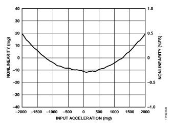
Figure 8. Z-Axis Nonlinearity, ±2 g Input Range
