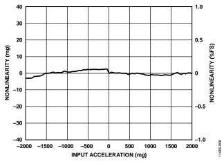
Figure 6. X-Axis Nonlinearity, ±2 g Input Range
