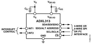
Figure 23. Application Diagram
