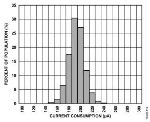
Figure 13. Current Consumption, Measurement Mode, Data Rate = 100 Hz,  $V_S = V_{DDVO} = 3.3 \text{ V}, 25^{\circ}\text{C}$
