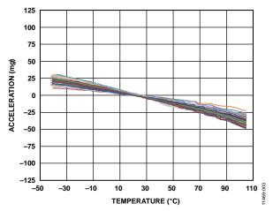
Figure 3. X-Axis Acceleration vs. Temperature, Three Lots (N = 80)
