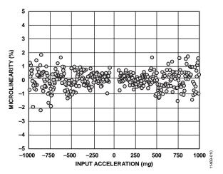
Figure 10. Y-Axis Microlinearity, 50 mg Step Size
