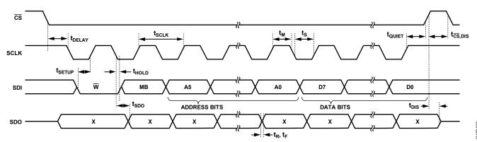
Figure 19. SPI 4-Wire Write
