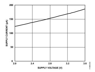
Figure 14. Supply Current vs. Supply Voltage, V₅ at 25°C
