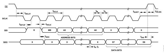
Figure 18. SPI 4-Wire Read
