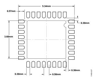
Figure 31. Sample Solder Pad Layout (Land Pattern)
