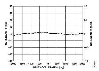
Figure 7. Y-Axis Nonlinearity, ±2 g Input Range
